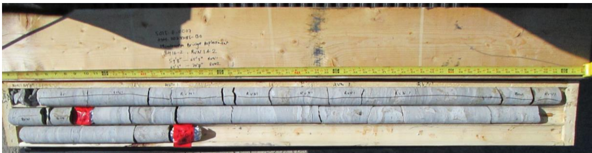
Photo 2. Core Sample for BH 16-2 from Elevation 159.4 m to 156.2 m
