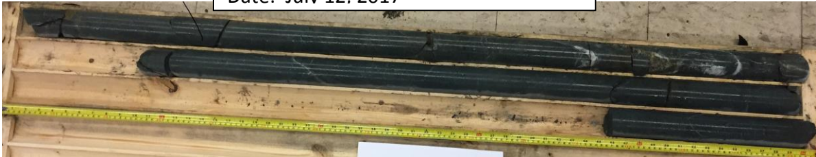
Photo 4. Bedrock Core Sample for BH5 from Elevation 302.3 m to 299.2 m
