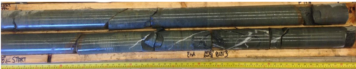
Photo 7. Bedrock Core Sample for BH8 from Elevation 309.2 m to 306.2 m
