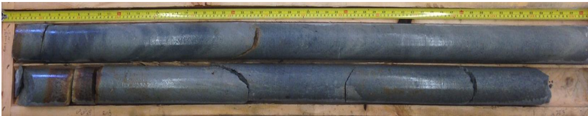
Photo 6. Bedrock Core Sample for BH7 from Elevation 307.9 m to 304.8 m
