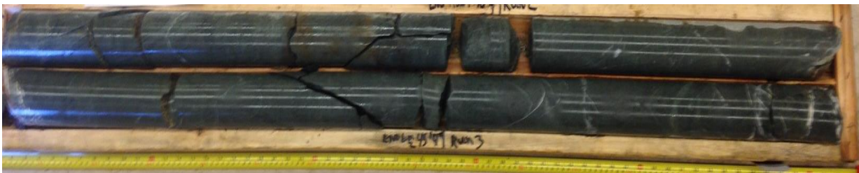
Photo 2. Bedrock Core Sample for BH2 from Elevation 302.3 m to 299.2 m
