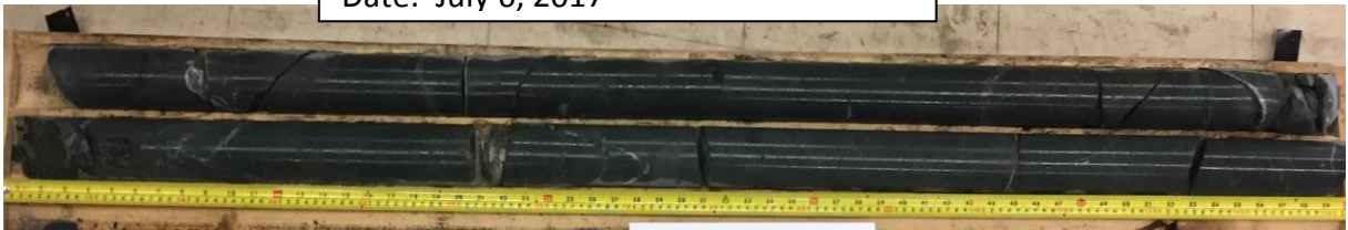
Photo 5. Bedrock Core Sample for BH6 from Elevation 303.2 m to 300.2 m
