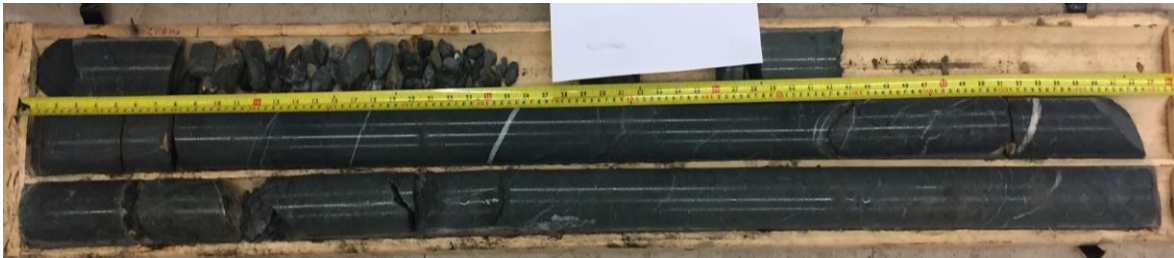
Photo 1. Bedrock Core Sample for BH1 from Elevation 302.0 m to 298.8 m
