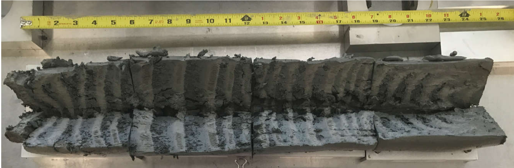
Photo C1. Shelby tube sample ST14 @ 15.2 to 15.9 m from Borehole 16-4
