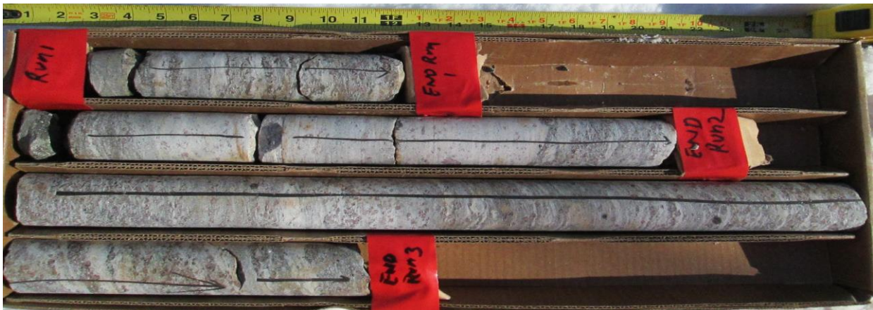
Figure E1. Rock cores from BH F15-2 - from Elev. 315.3 m to 313.3 m
