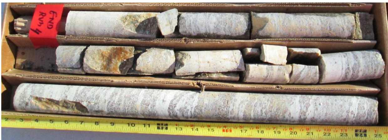
Figure E2. Rock cores from BH F15-2 - from Elev. 313.3 m to 311.7 m
