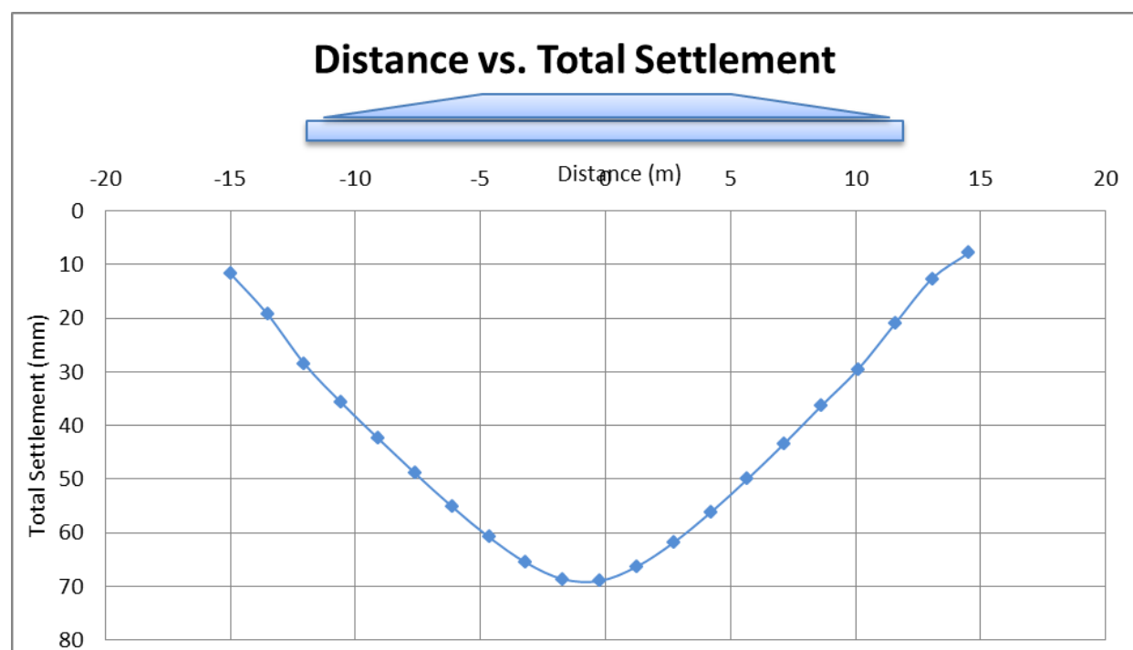
Figure G4. Settlement result for footing on 2m of engineered fill
