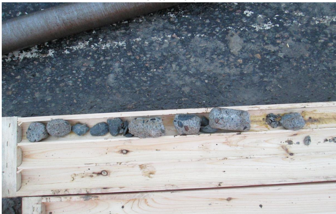
Photo 14. Core sample recovered from BH-2A at Elevation 251.0 m to 250.8 m
