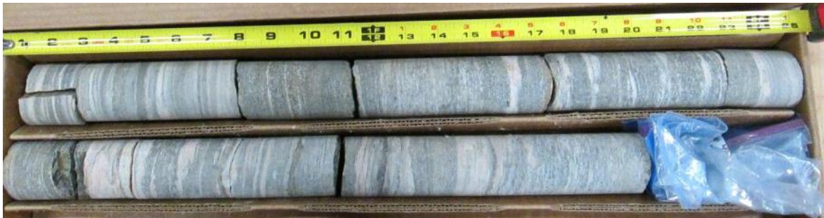
Photo 1. Core Sample for BH1 from Elevation 336.0 m to 334.85 m
