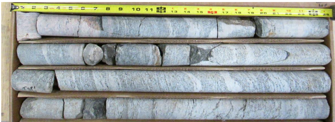
Photo 2. Core Sample for BH1 from Elevation 334.85 m to 332.0 m
