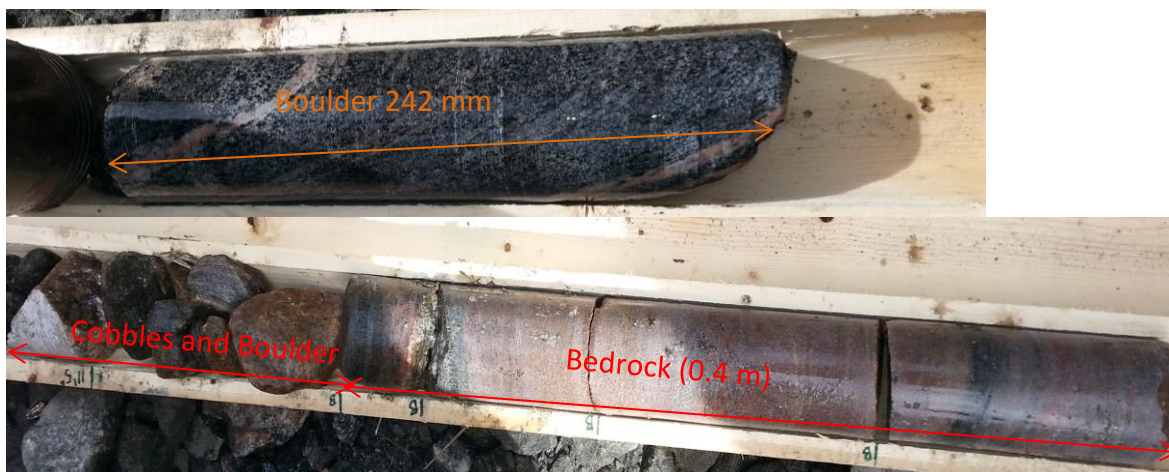
Photo 6. Core Sample for BH7A from Elevation 255.7 m to 253.9 m
