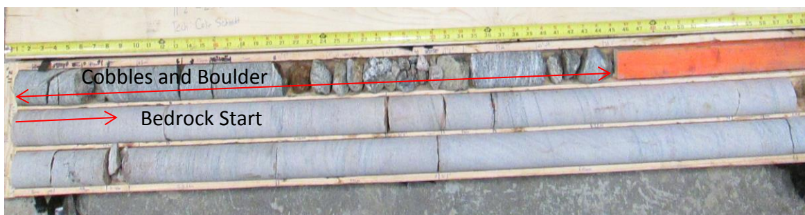
Photo 4. Core Samples BH6 Cobbles and Boulders from Elevation 255.8 m to 251.8 m and Bedrock from Elevation 251.8 m to 248.9 m
