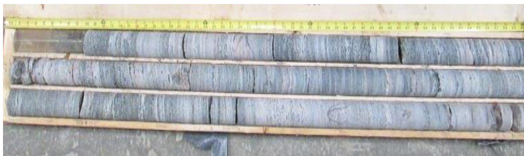
Photo 2. Core Sample for BH3 from Elevation 243.4 m to 238.9 m
