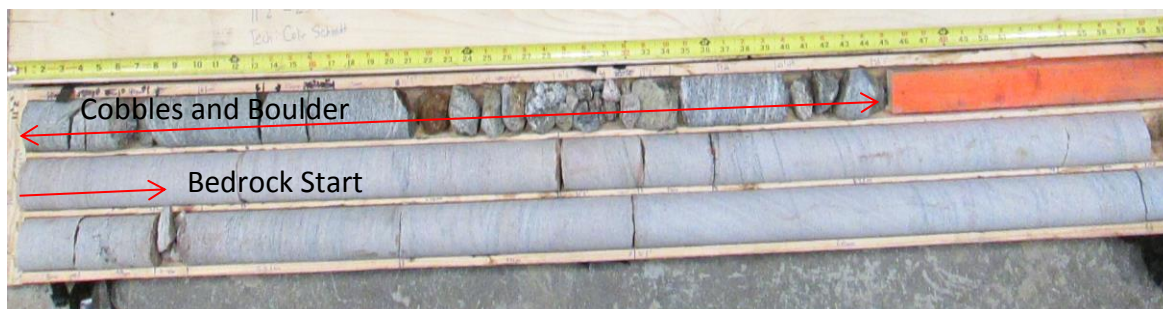
Photo 4. Core Samples BH6 Cobbles and Boulders from Elevation 255.8 m to 251.8 m and Bedrock from Elevation 251.8 m to 248.9 m
