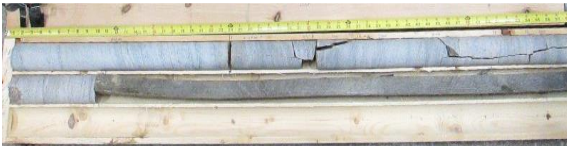
Photo 5. Core Sample for BH6 from Elevation 248.9 m to 247.2 m
