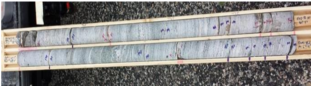
Photo 1. Core Sample for BH1 from Elevation 241.3 m to 238.3 m
