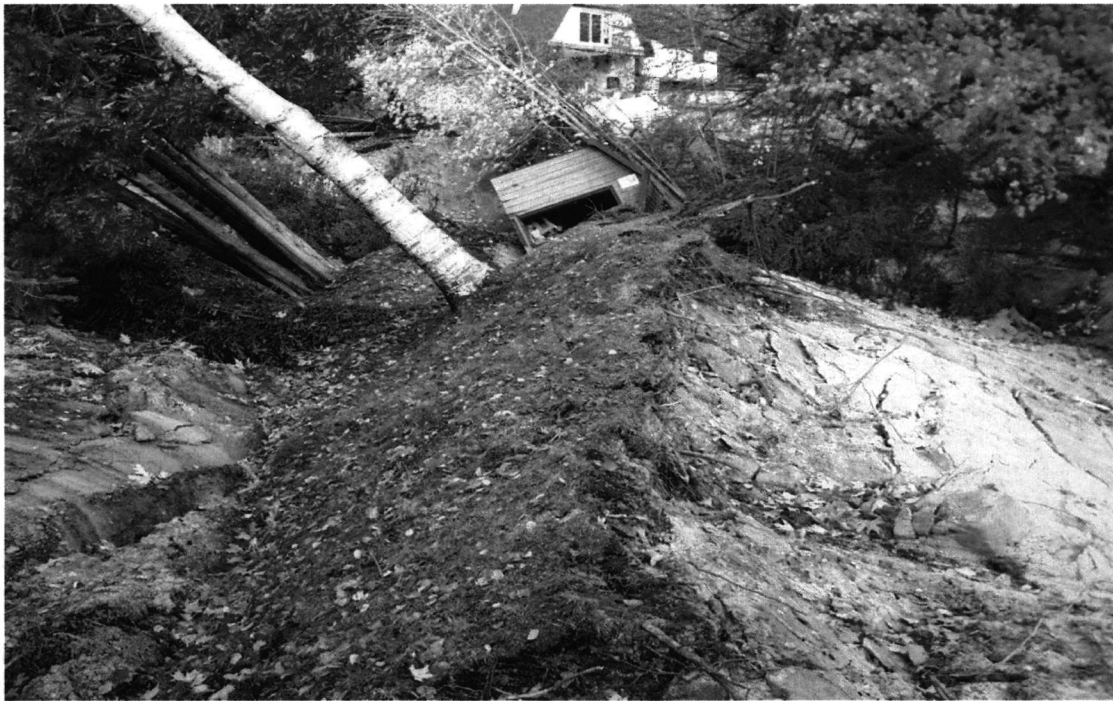
Photo 1 – Sectional View of Compound Failure. Note concentric slips dipping backwards.
