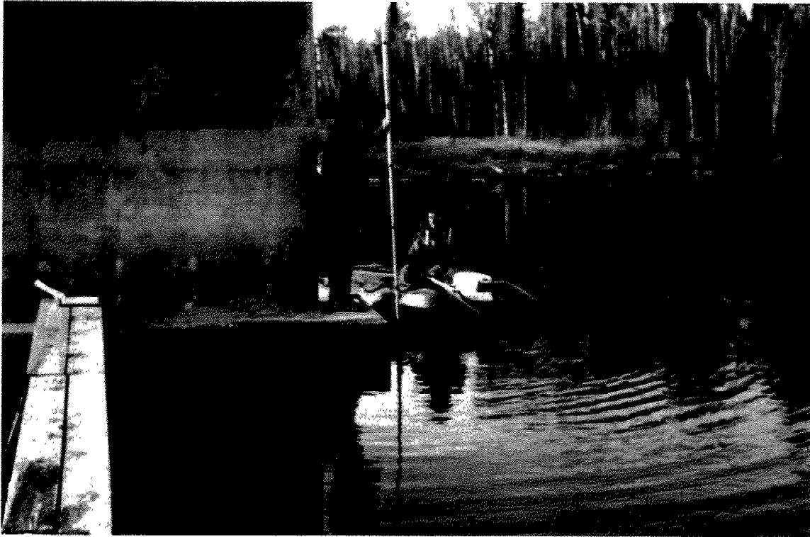
PHOTOGRAPH 3 Obtaining water depth soundings around bridge pier.
