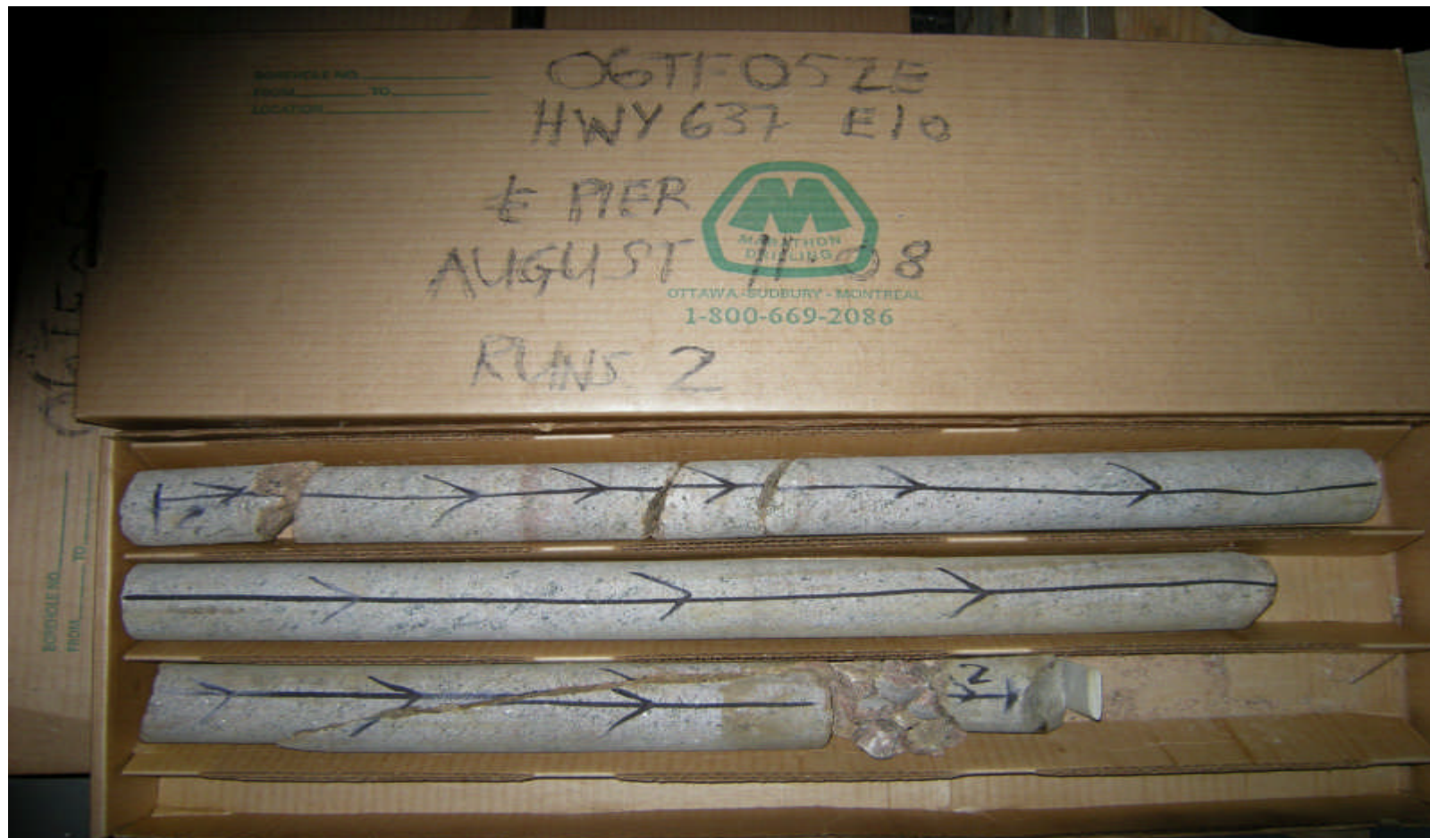
Centre Pier Core Photograph 3: Rock core from borehole E10 - RC-2 and RC-3
