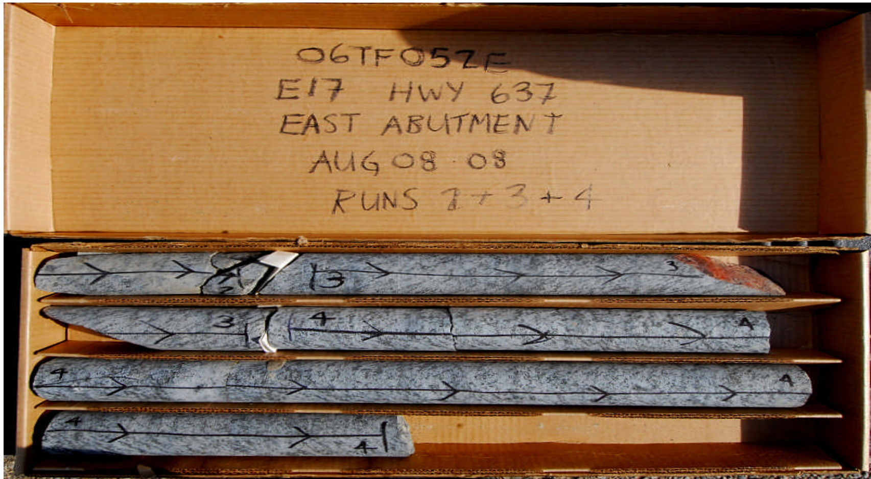
East Abutment Core Photograph 6: Rock core from borehole E17, bottom of RC-6, RC-7 and RC-8
