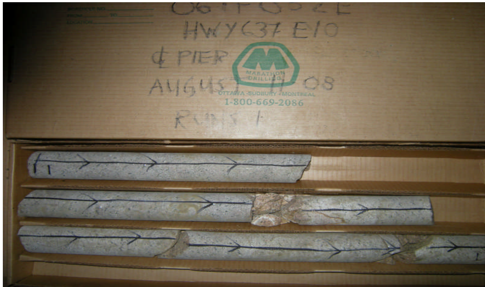
Centre Pier Core Photograph 2 : Rock core from borehole E10 - RC-1
