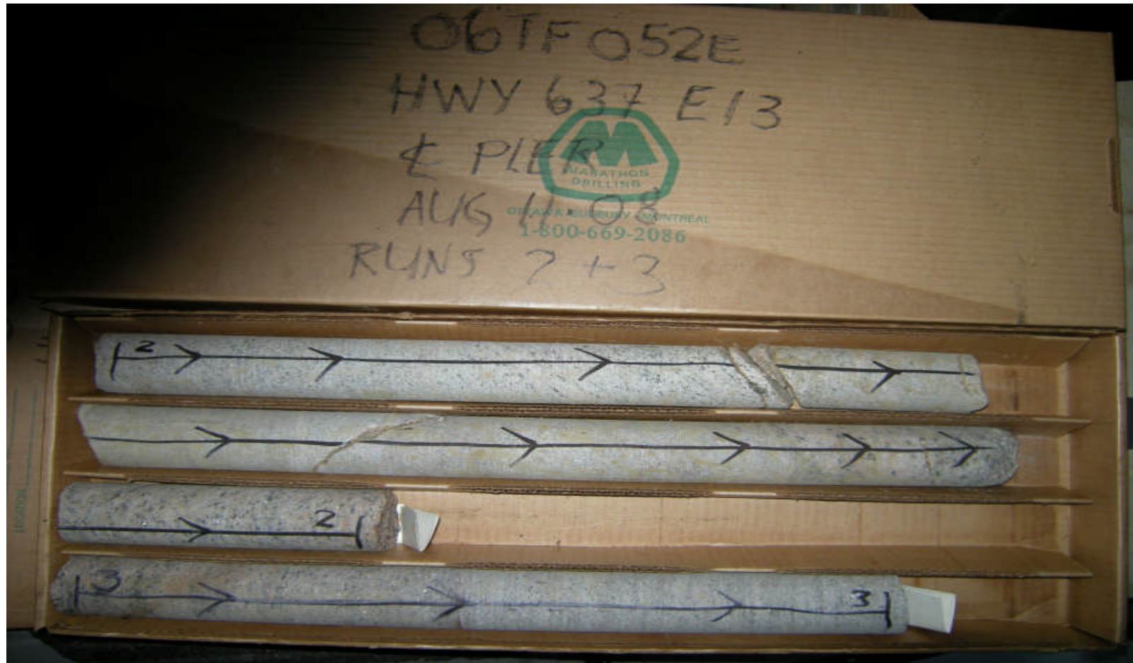
Centre Pier Core Photograph 6: Rock core from borehole E13 - RC-2 and RC-3
