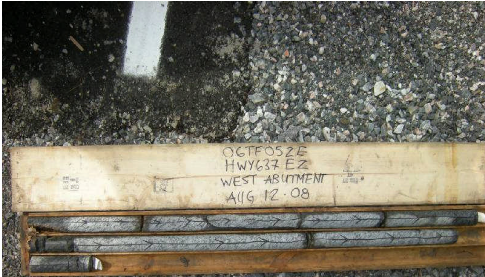
West Abutment Core Photograph 1 : Rock core from borehole E2 - RC-1 and RC-2
