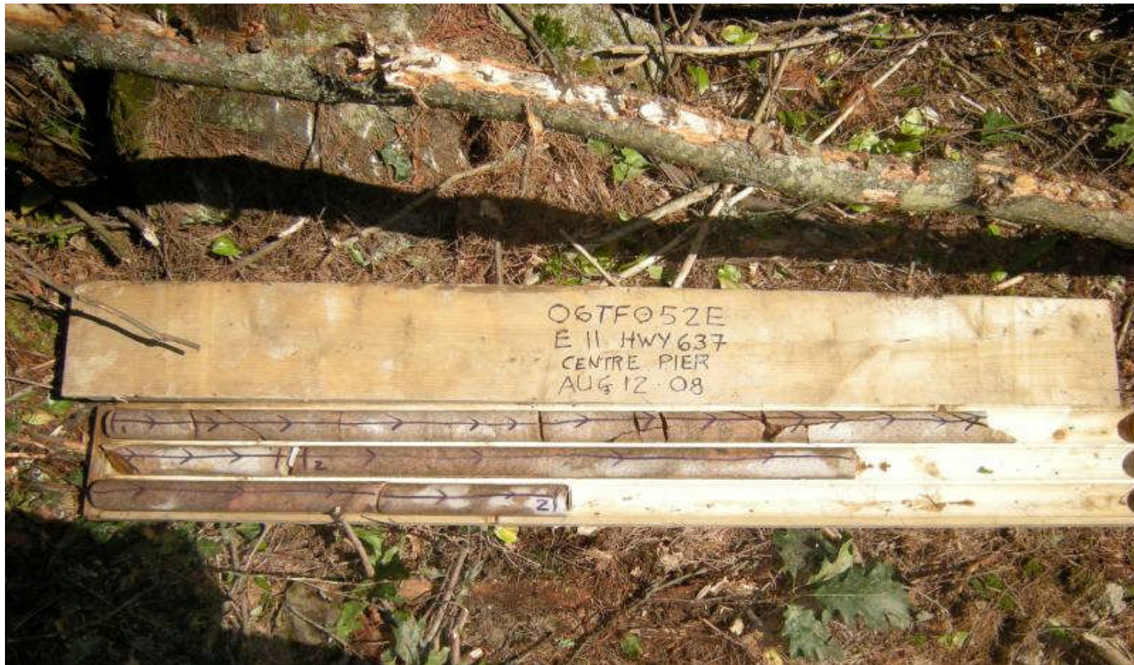
Centre Pier Core Photograph 4: Rock core from borehole E11 - RC-1 and RC-2
