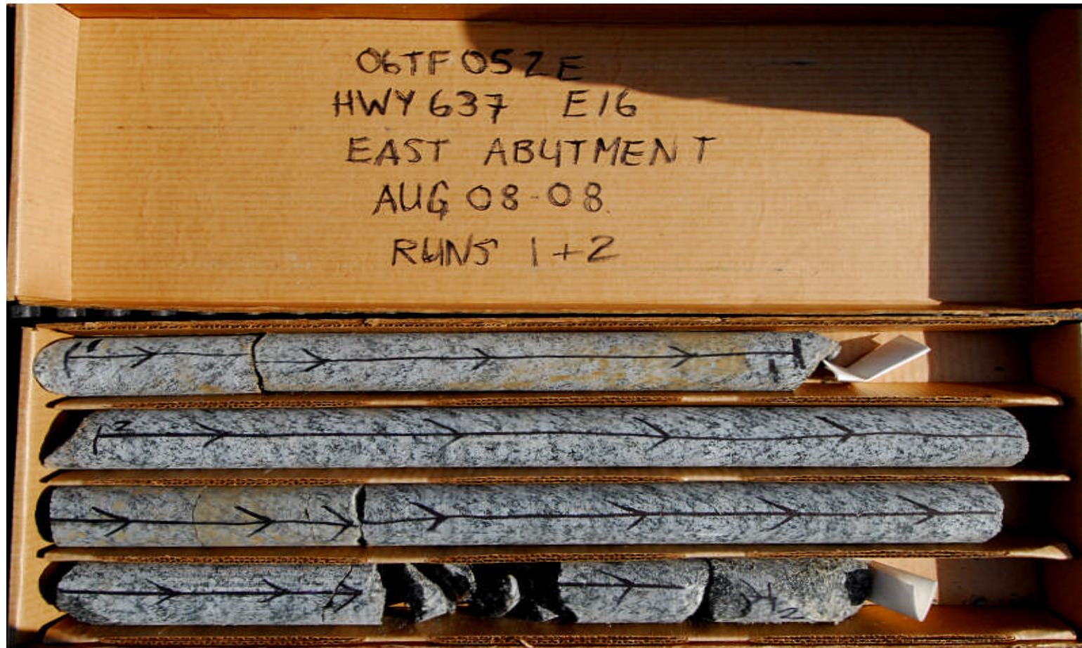
East Abutment Core Photograph 3: Rock core from borehole E16 - RC-5 and RC-6
