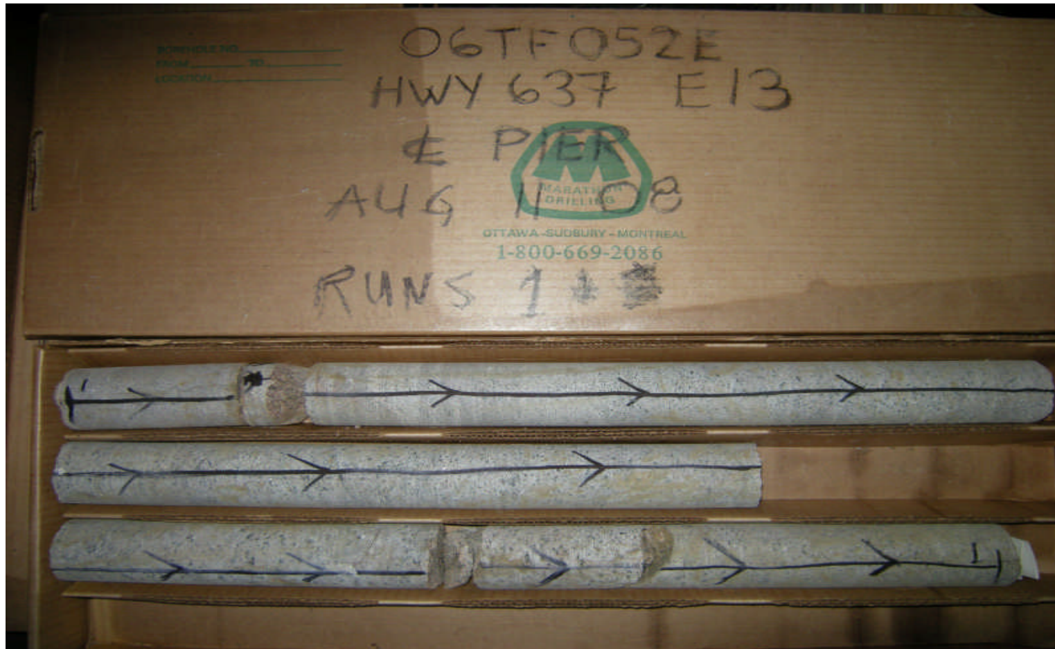
Centre Pier Core Photograph 5: Rock core from borehole E13 - RC-1
