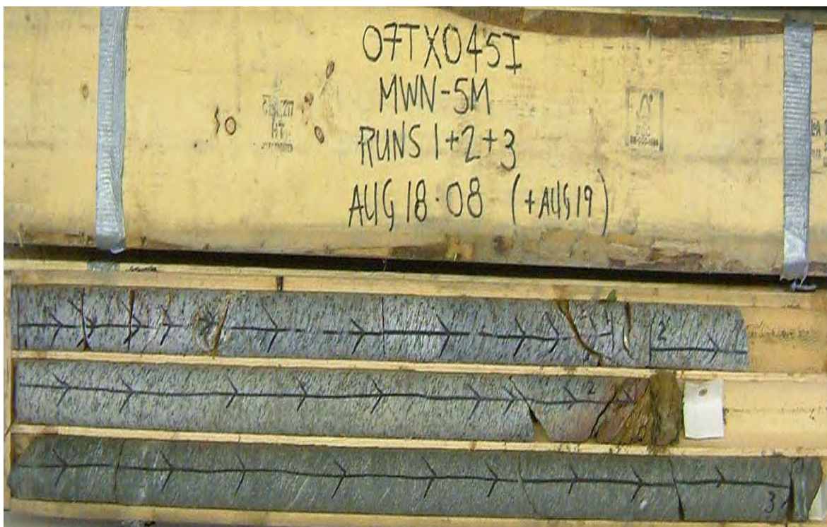
Core Photo 14: Borehole N5M, Run 1 to 3, 0.8 to 4.6 m.
