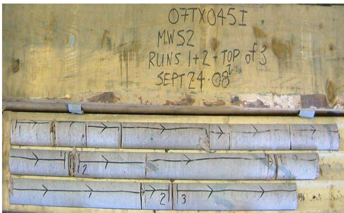
Core Photo 2: Borehole S2, Run 1 to 3, 0.0 to 4.2 m.
