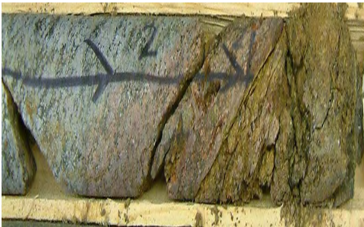
Core Photo 15: Borehole N5M, Close up view of Run 2 showing oxidation and weathering.
