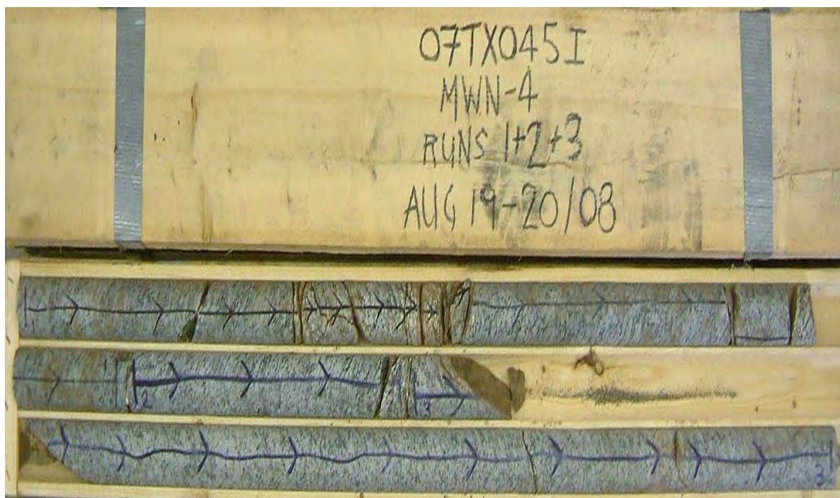
Core Photo 9: Borehole N4, Run 1 to 3, 0.0 to 3.7 m.
