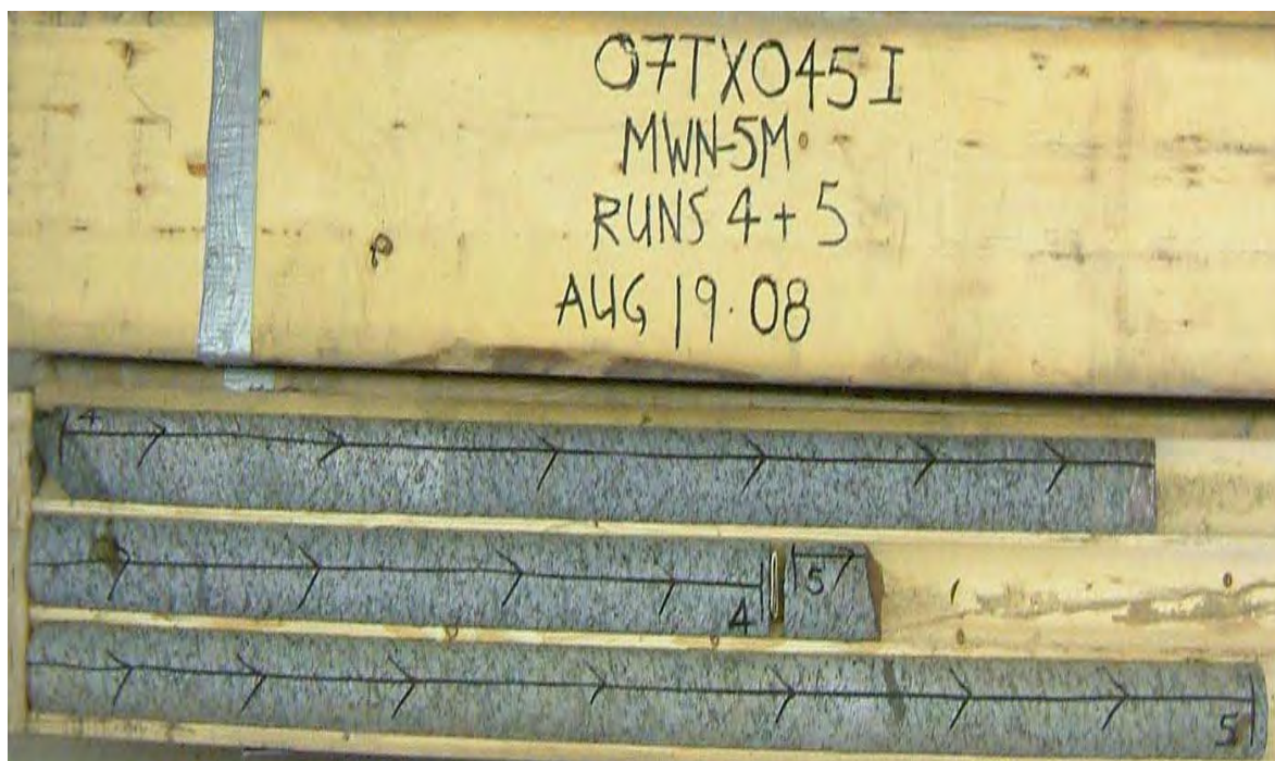
Core Photo 16: Borehole N5M, Run 4 and 5, 4.6 to 7.7 m.
