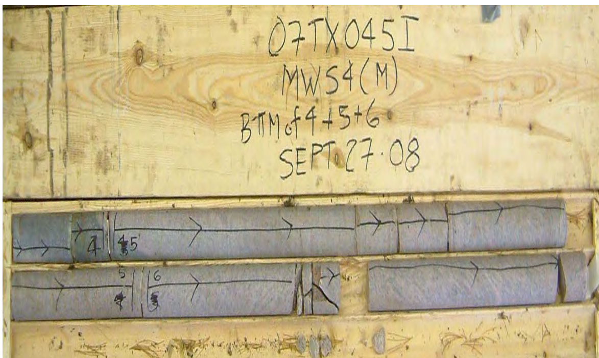
Core Photo 10: Borehole S4M, Run 5, 6 and bottom part of Run 4, 4.6 to 7.4 m.
