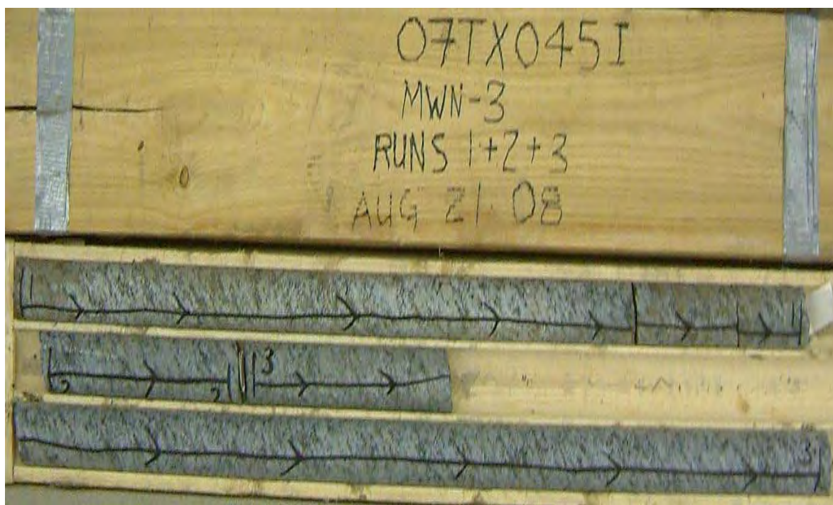
Core Photo 7: Borehole N3, Run 1 to 3, 0.0 to 3.2 m.
