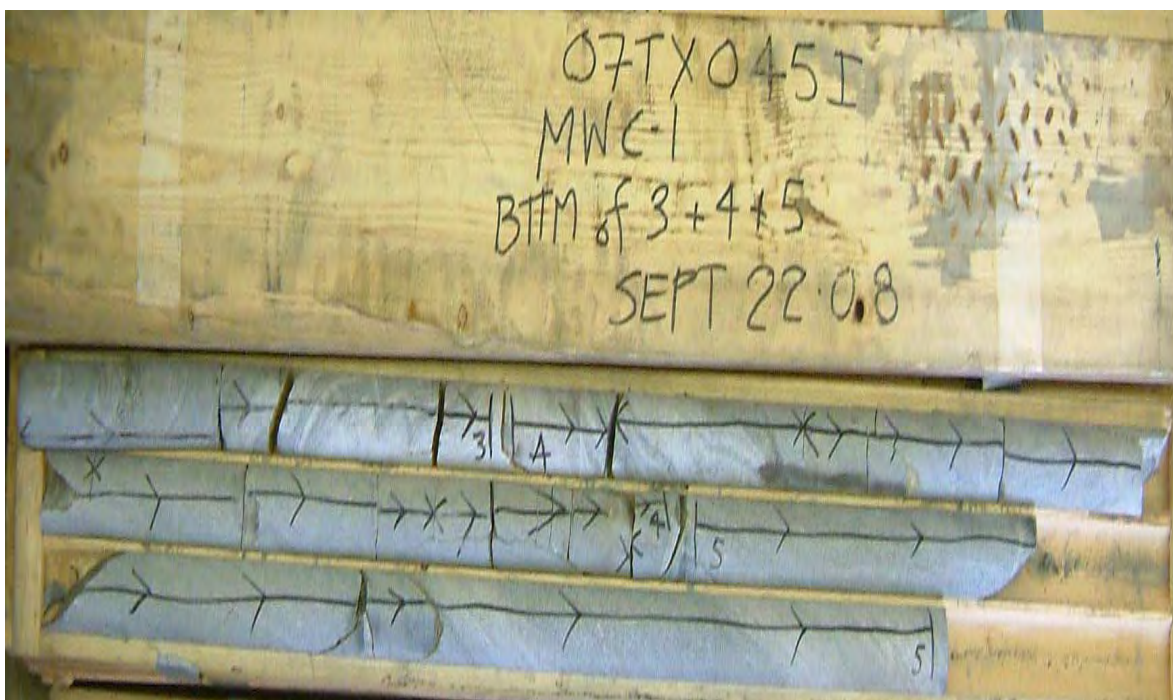
Core Photo 2: Borehole C1, Run 4, 5 and bottom part of Run 3, 2.7 to 7.8 m.
