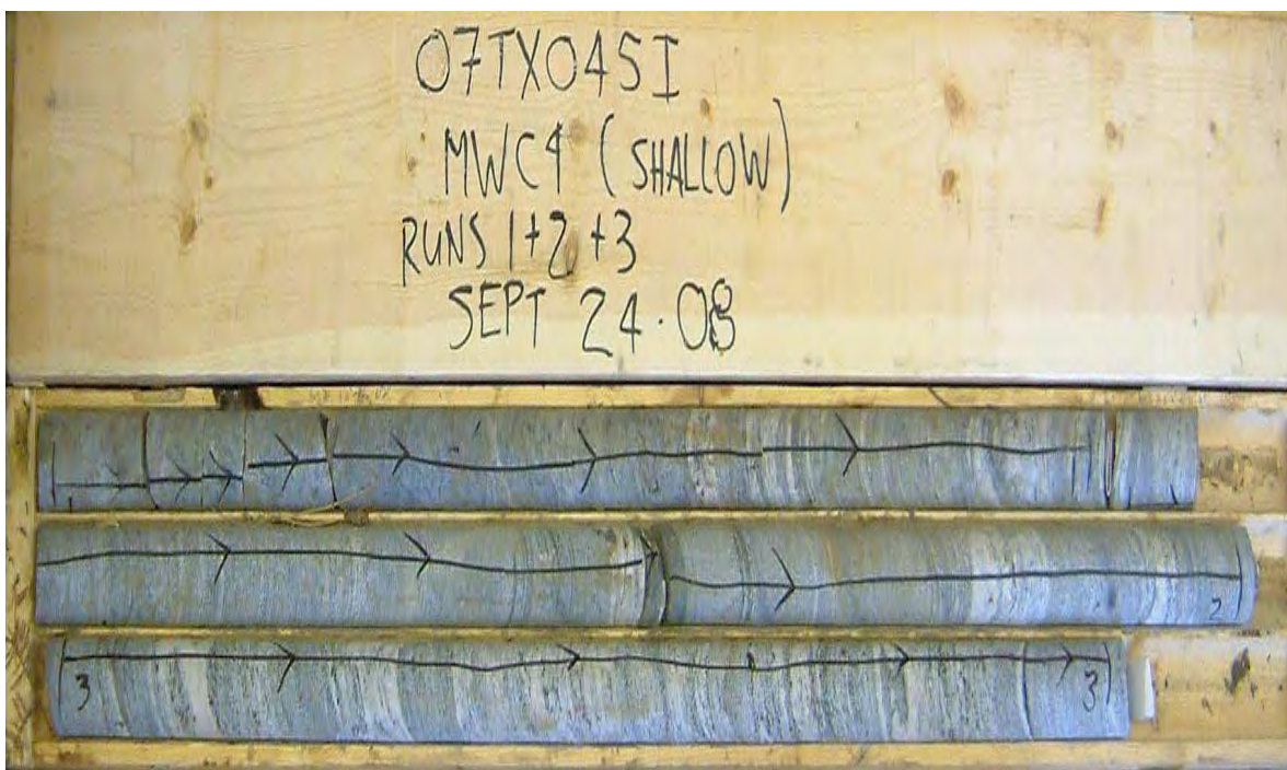
Core Photo 12: Borehole C4S, Run 1 to 3, 0.6 to 4.7 m.
