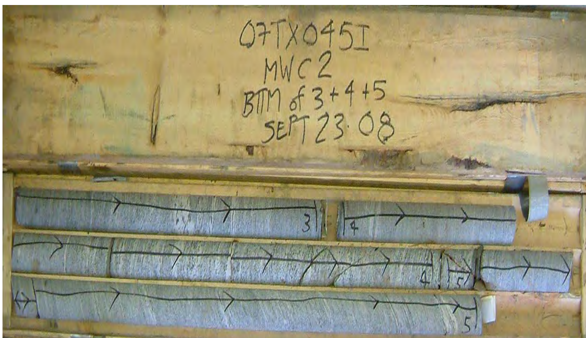
Core Photo 4: Borehole C2, Run 4, 5 and bottom part of Run 3, 4.0 to 7.6 m.
