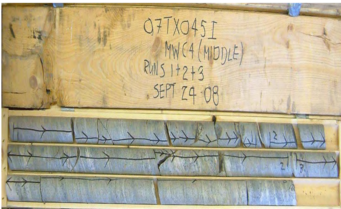
Core Photo 10: Borehole C4M, Run 1 to 3, 0.7 to 4.9 m.
