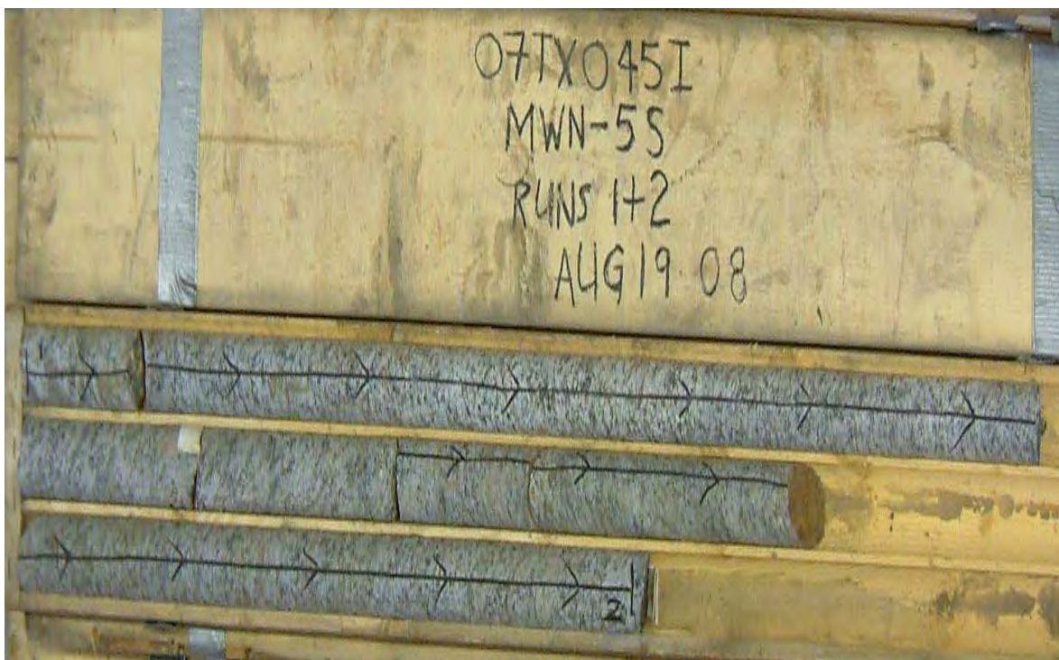
Core Photo 17: Borehole N5S, Run 1 and 2, 0.2 to 3.3 m.
