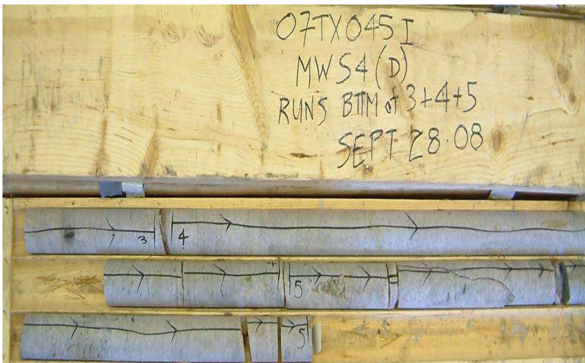
Core Photo 7: Borehole S4D, Run 4, 5 and bottom part of Run 3, 4.5 to 7.8 m.
