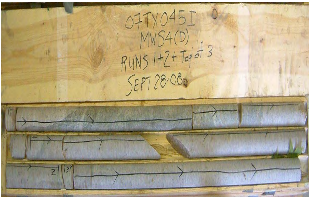
Core Photo 6: Borehole S4D, Run 1 to 3, 0.1 to 4.5 m.
