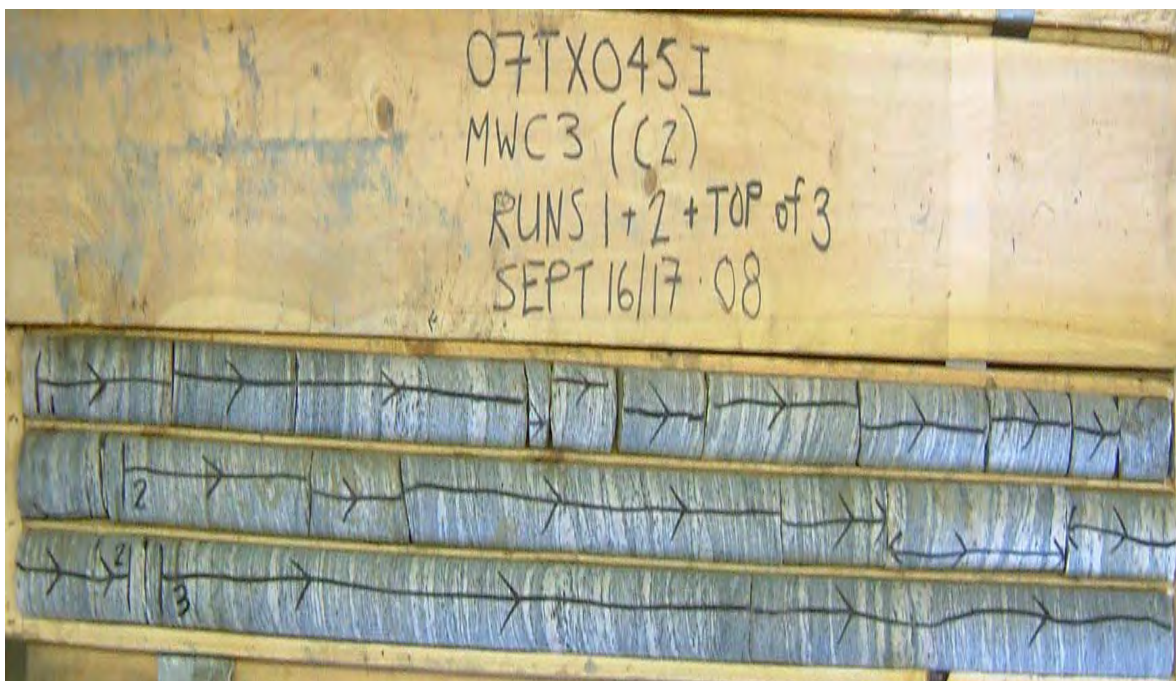
Core Photo 5: Borehole C3, Run 1 to 3, 0.0 to 4.5 m.
