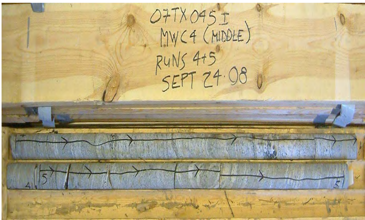
Core Photo 11: Borehole C4M, Run 4 and 5, 4.9 to 7.8 m.
