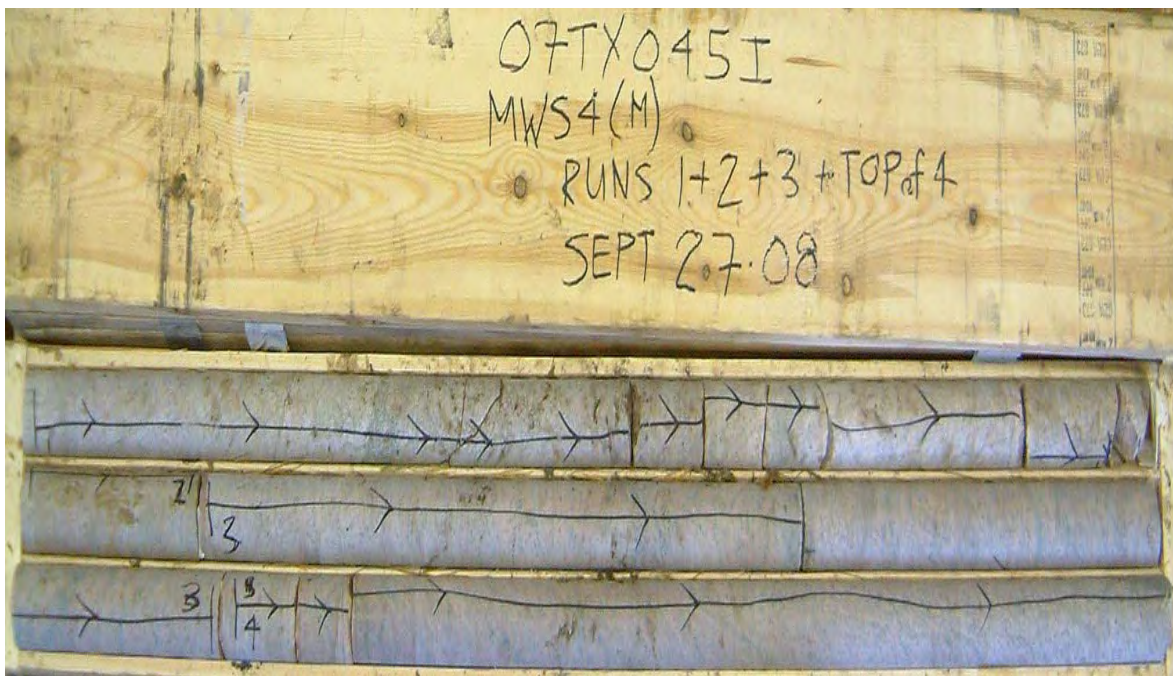
Core Photo 9: Borehole S4M, Run 1 to 4, 4.0 to 4.6 m.
