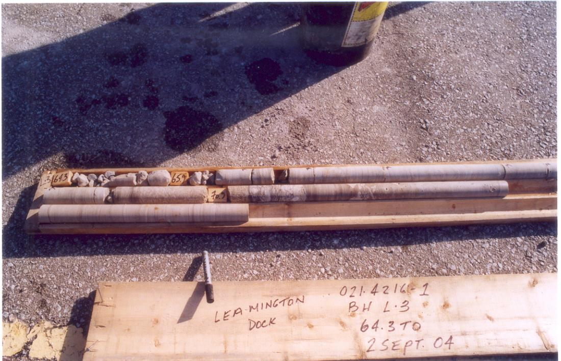
Photo 2: Rock core from borehole 103.
