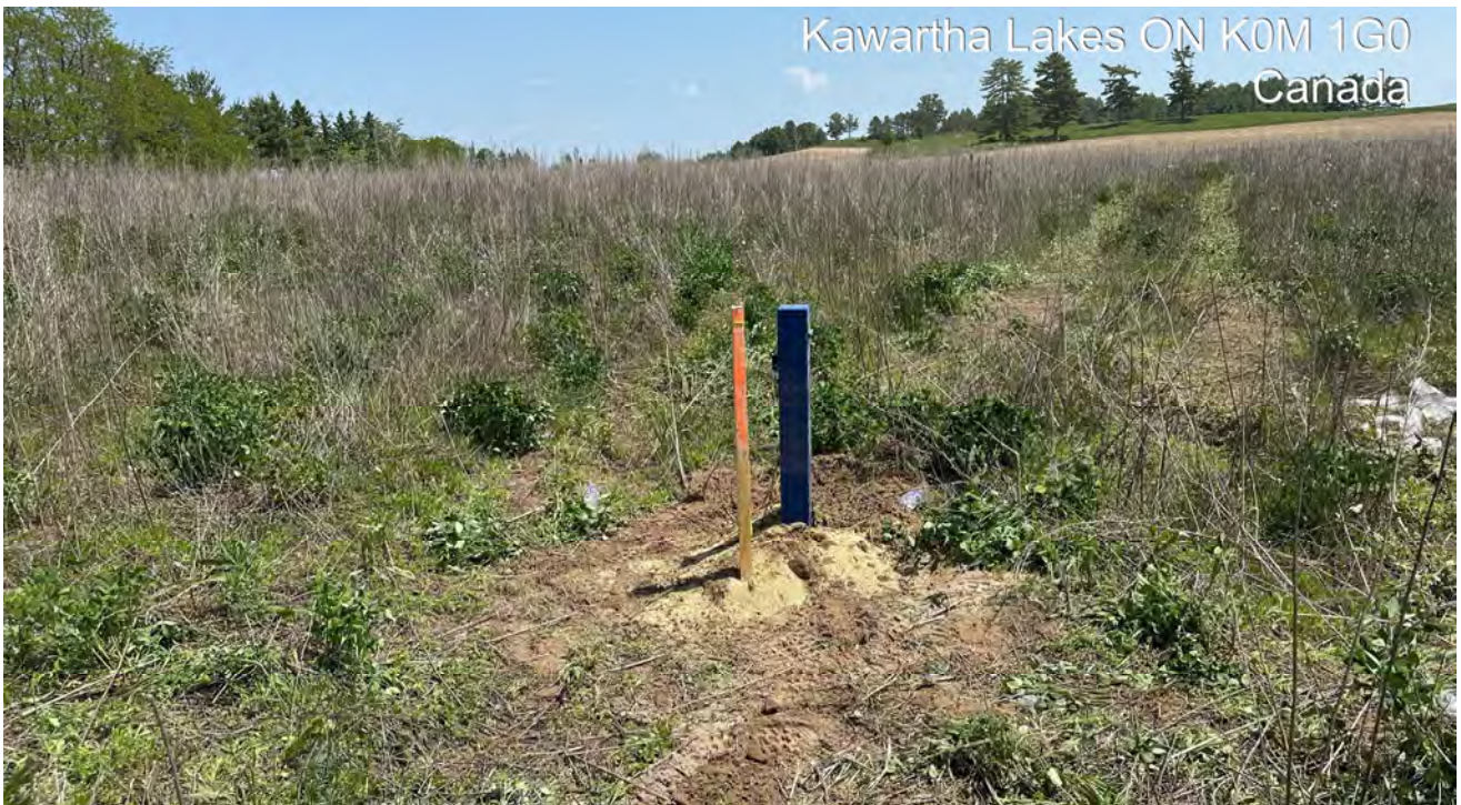
Photograph #4 – Looking east. Monitoring well is installed in the area of the proposed underground water storage tanks (Borehole FST-01).
