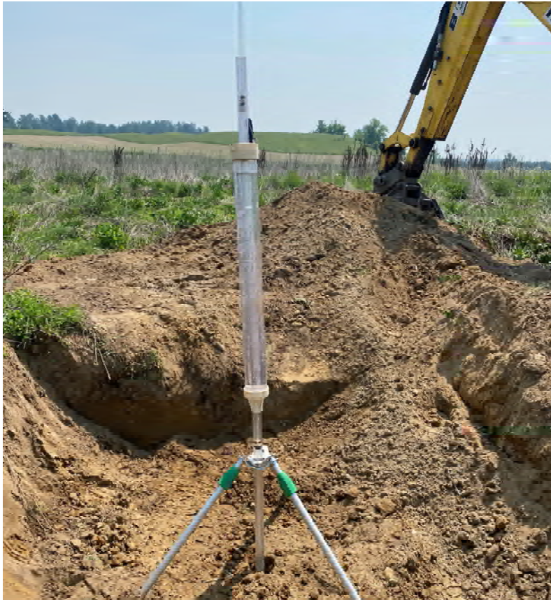
Photograph #5 – Test pit excavation to perform in-situ infiltration (Guelph permeameter) test at the proposed stormwater management pond location (Test Pit TP-01).
