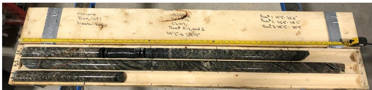
Photo C2: Borehole 22-02 Bedrock Core Sample (Runs 1, 2 and 3)
