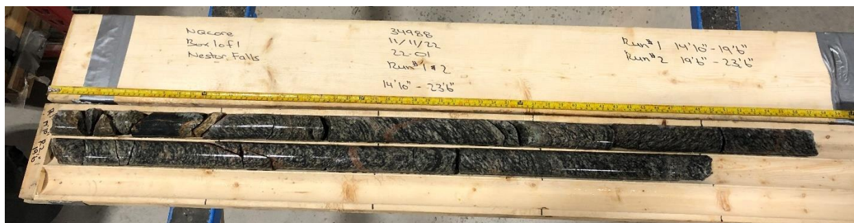
Photo C1: Borehole 22-01 Bedrock Core Sample (Runs 1 and 2)
