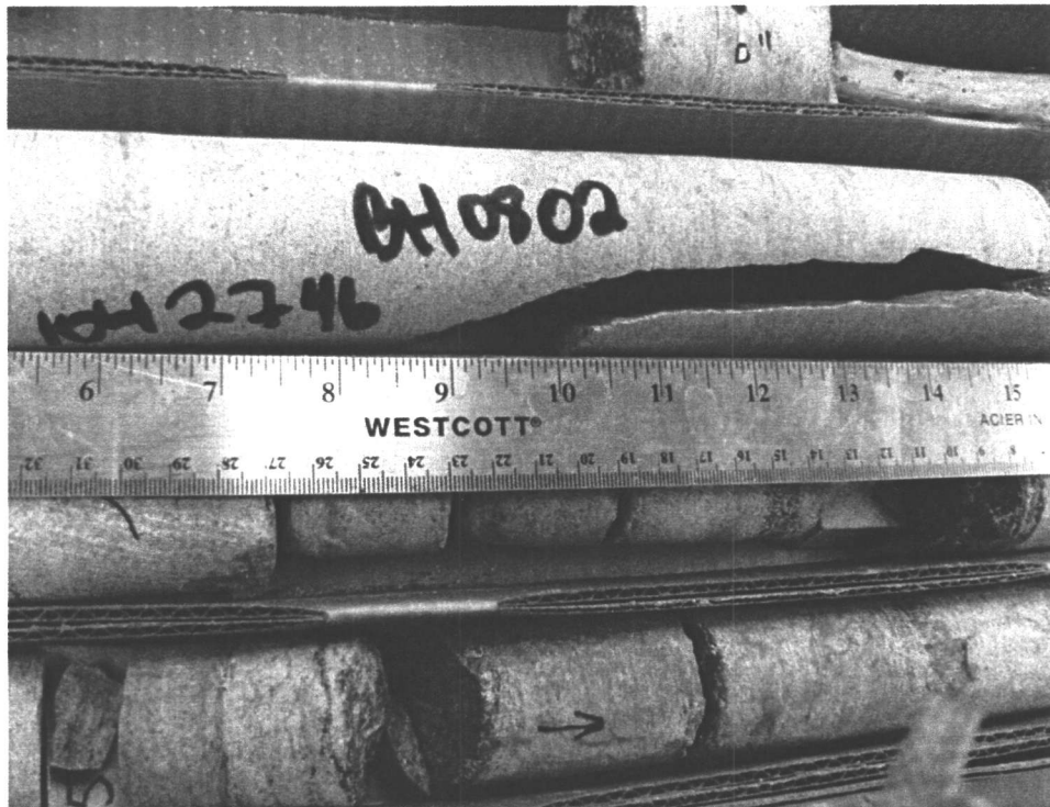
Photo 3: BH08-2 Vertical fracture in bedrock core
