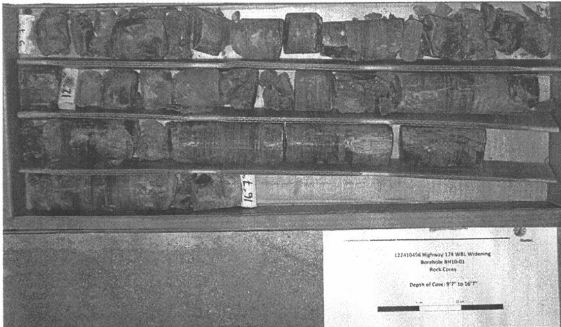
Photo No. 1: Bedrock core from borehole BH10-01 (2.9 m to 5.1 m)
