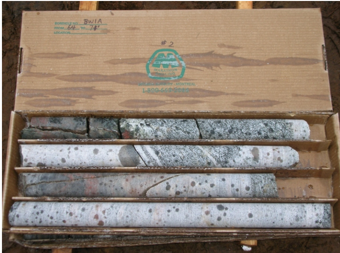
Photograph #14 View of core and fissures in the core taken from 19.2m to 21.3m of Well EBW 14.
