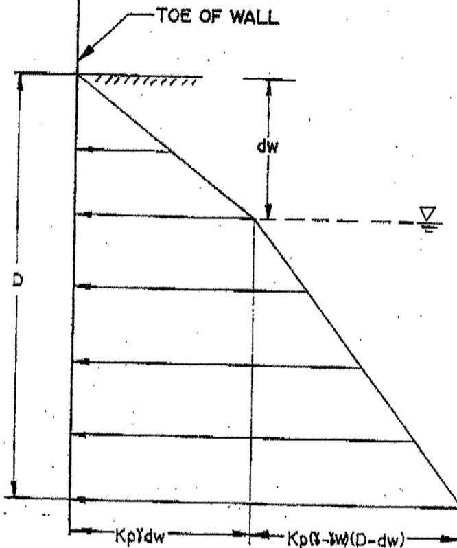
$K_p$  = COEFFICIENT OF PASSIVE EARTH PRESSURE
