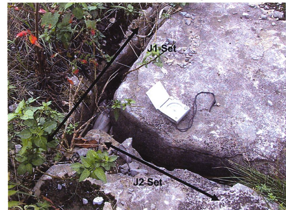
C) Close-Up of Typical Near-Surface Open Jointing
