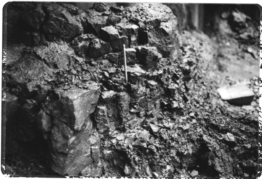
Photo No. 15 - Close up of rock bench along east wall to cell showing thin clay seam at pencil tip.
