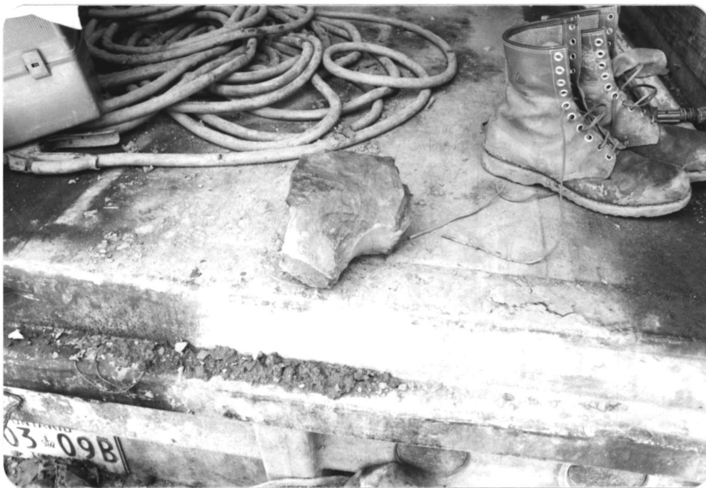
Photo No. 22 - Rock fragment taken by contractor at approximately elevation 255 feet showing borehole edge.
