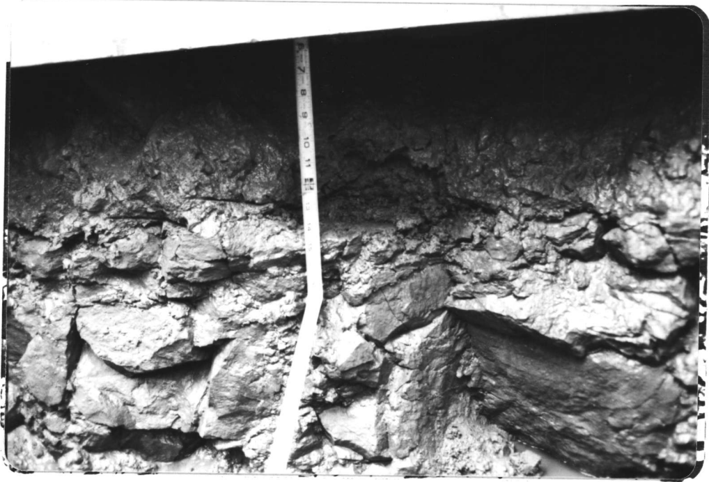
Photo No. 9 - Till overlying rock along south wall. Top of rock at approximately elevation 251 feet.
