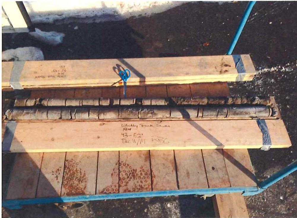
Photograph 1: Core Samples BH14-4 (43 – 52 ft depth).
