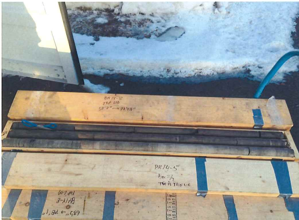
Photograph 2: Core Samples BH14-5 (55 – 70 ft depth).
