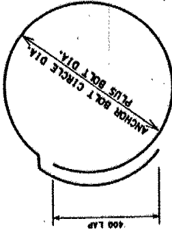
DETAIL OF 15M RINGS PLACED AT THE TOP. N.T.S.
