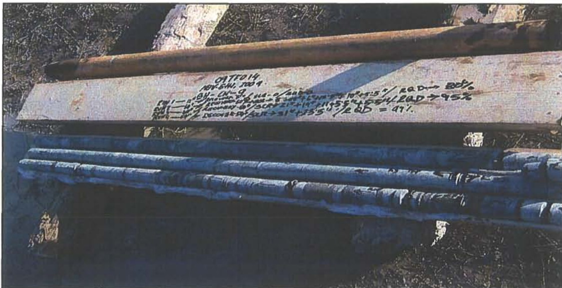
Photo 2: Rock cores retrieved from borehole CW-9, Core Runs 1 to 4 from 27.6 to 32.3 m depth. RQD of the rock cores ranges from 0 to 99%. The rock mass quality varies from very poor to excellent.
