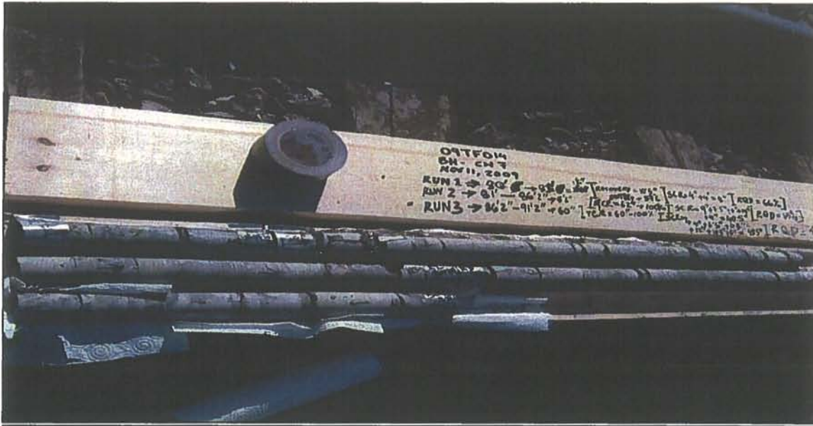
Photo 1: Rock cores retrieved from borehole CW-7, Core Runs 1 to 3 from 24.4 to 27.8 m depth. RQD of the rock cores ranges from 65 to 83%. The rock mass quality varies from fair to good.
