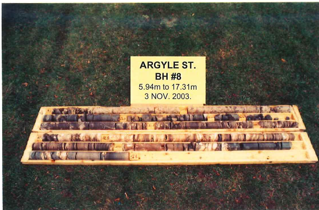
Photo 5 Borehole No. 8 – Rock core. Note concrete. Elevation 185.29m to 173.92m.
