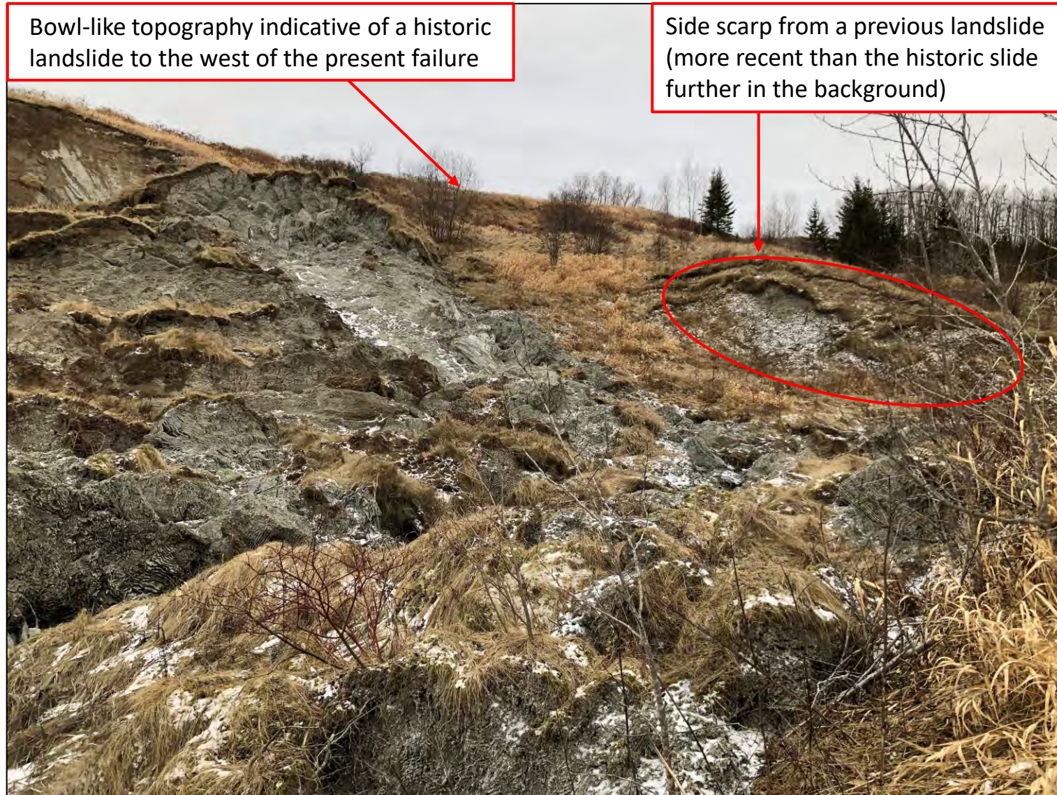
Photo 7: View looking southwest from the toe of the current failure showing the topography to the west, including a bowl-like topography indicative of a historic landslide and a more recent side scarp from a previous smaller-scale failure that likely overlapped the current failure. December 4, 2020
