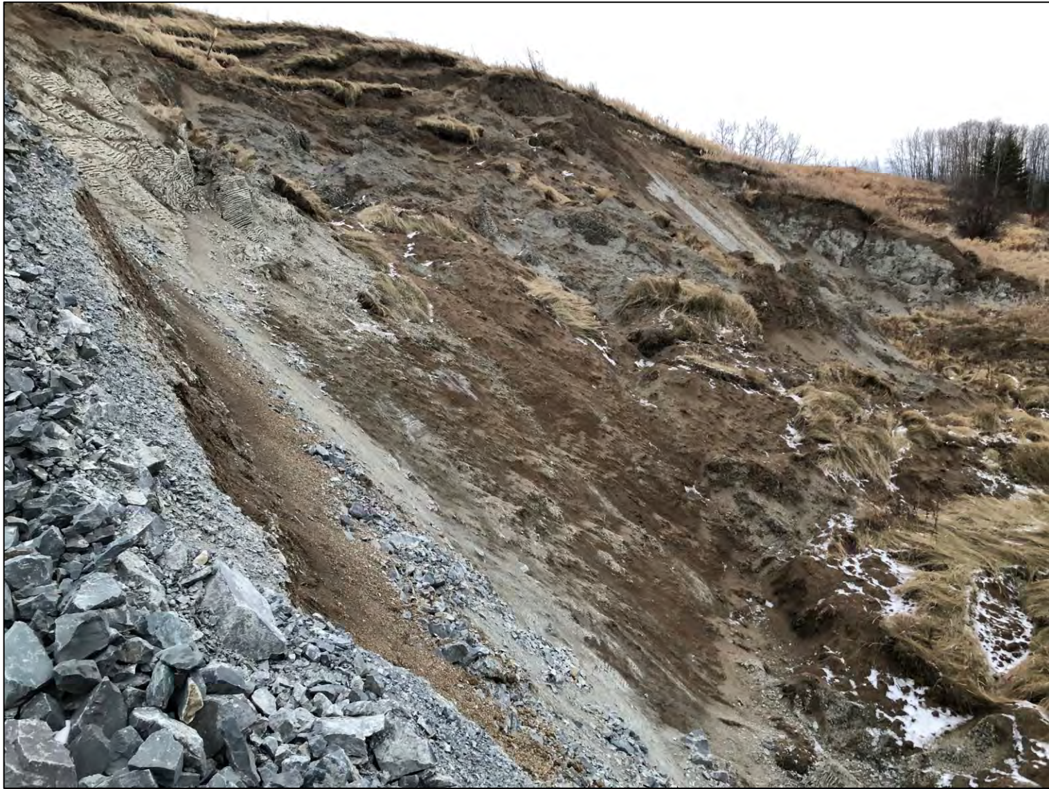
Photo 4: View of original slide scar, looking west, which is locally steeper with an angle of approximately 40 degrees. Retrogression can be seen above the original failure.
