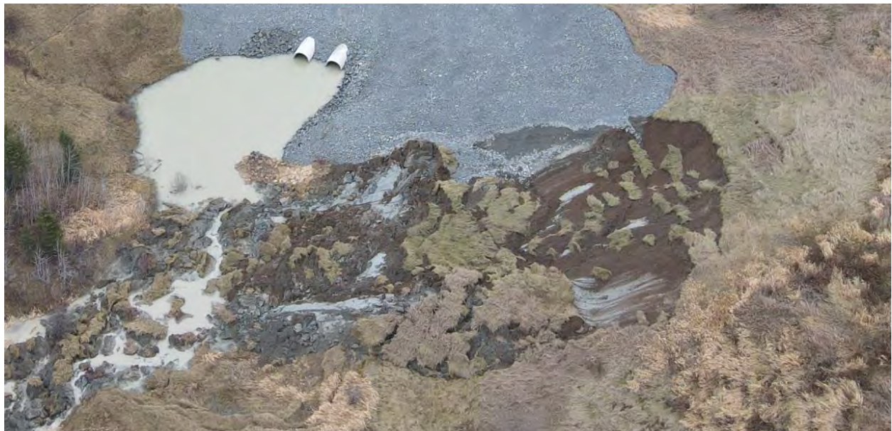
Figure 2: After Slope Failure
