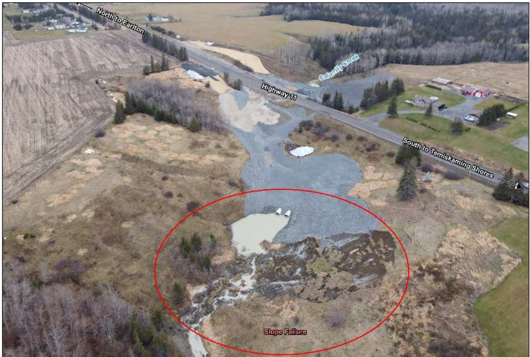
Photo 1: Aerial image from LGL Limited memo (dated November 18, 2020) showing the extent of the landslide on November 10, 2020. The head scarp of the slide has since retrogressed further to the southeast.
