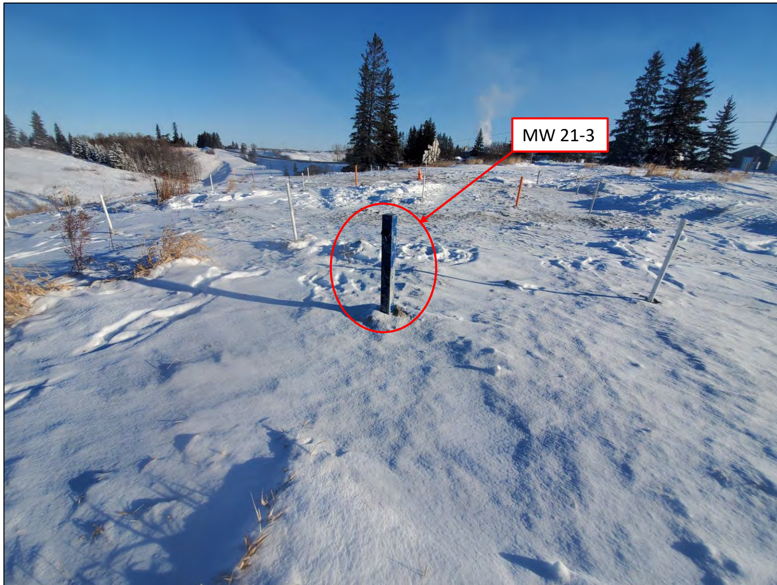
Photo 17: Monitoring well MW 21-3 installed in January, 2021.
