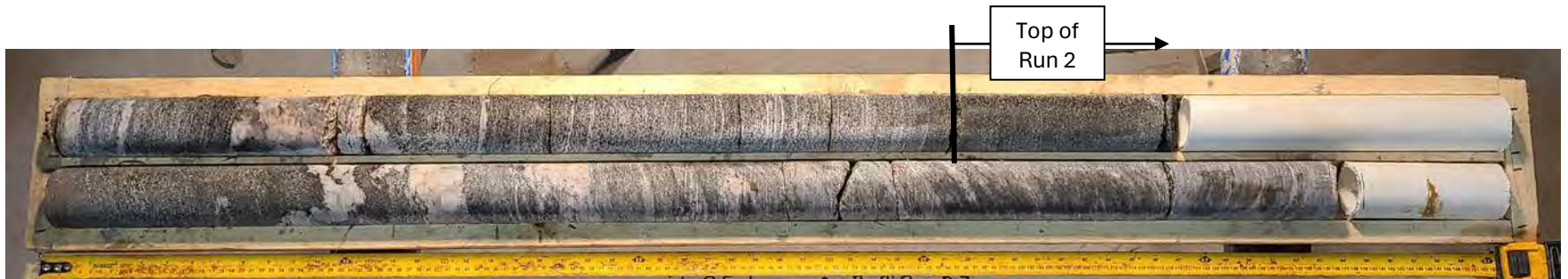
Borehole 23-02 – Runs 1 and 2 – 0.69 to 3.28 m
