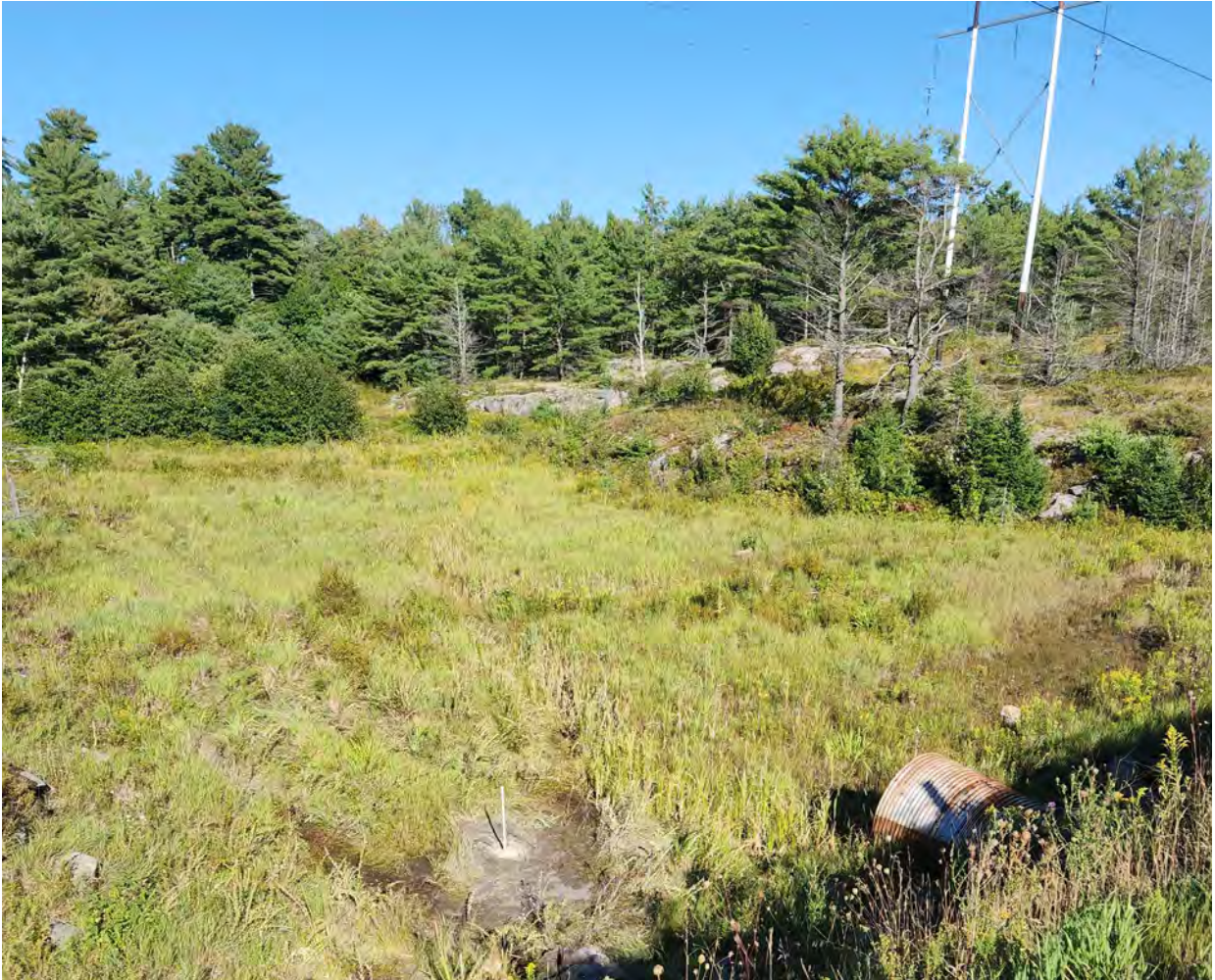
Photograph 3: Culvert Inlet with Piezometer at Borehole 23-01
