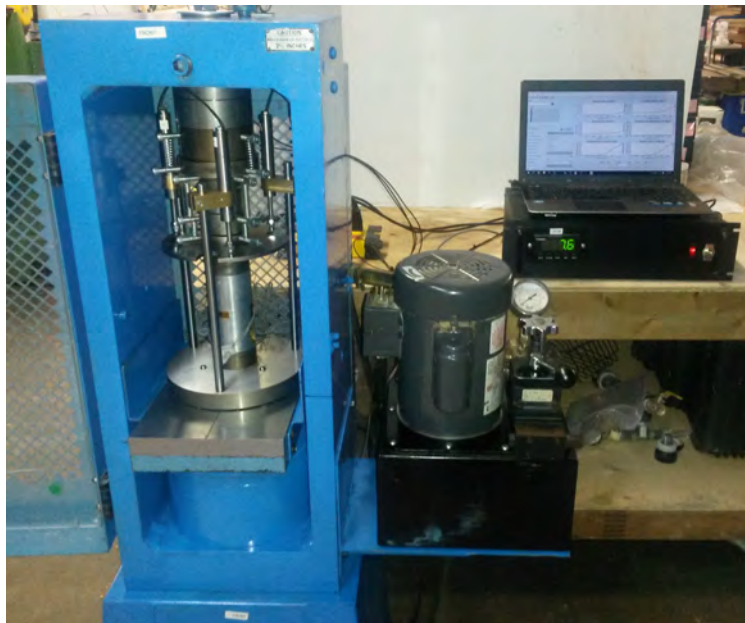
Figure 1: Forney loading frame setup for UCS testing.
