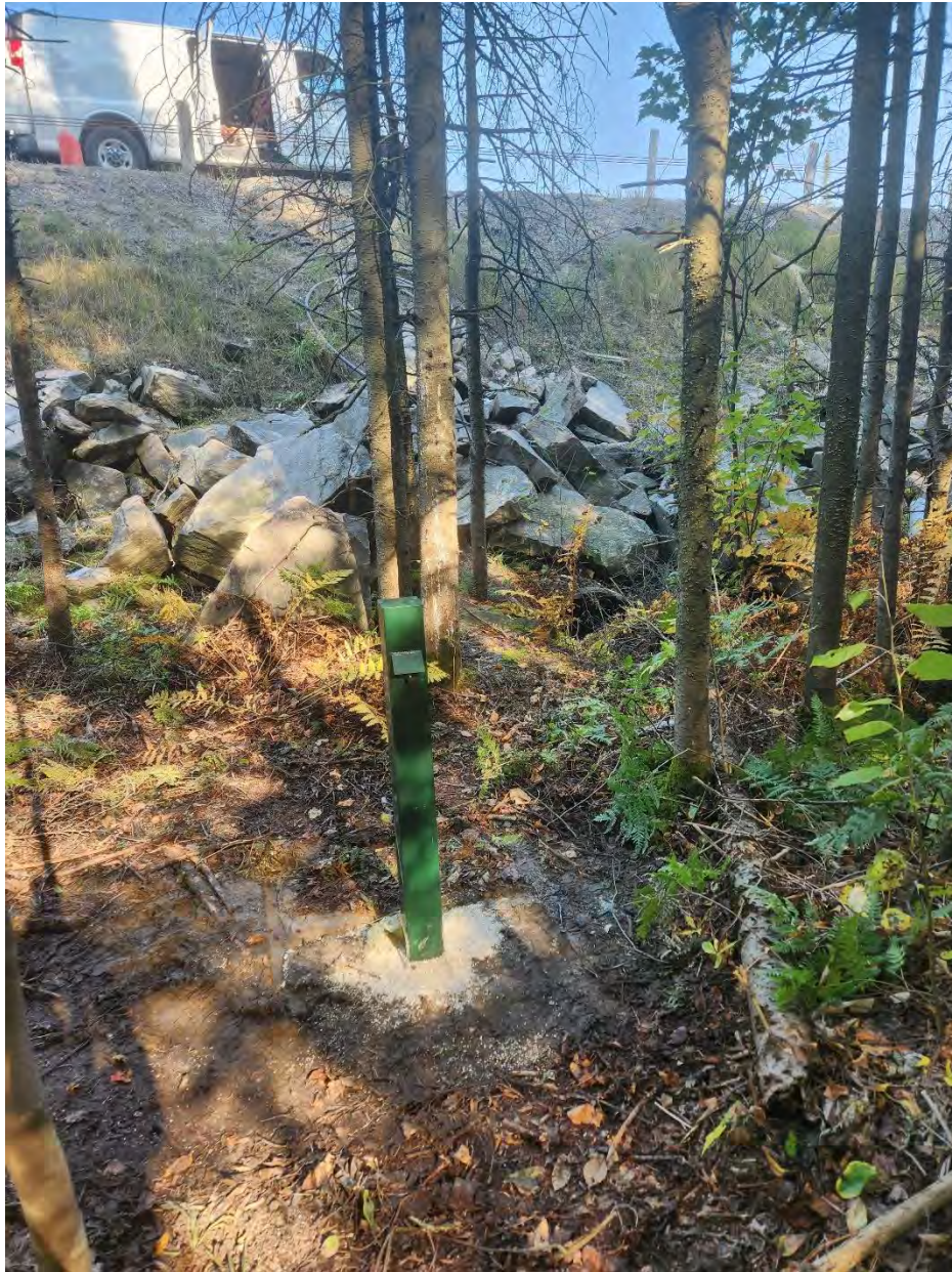
Photograph 5: Borehole 23-09 After Completion
