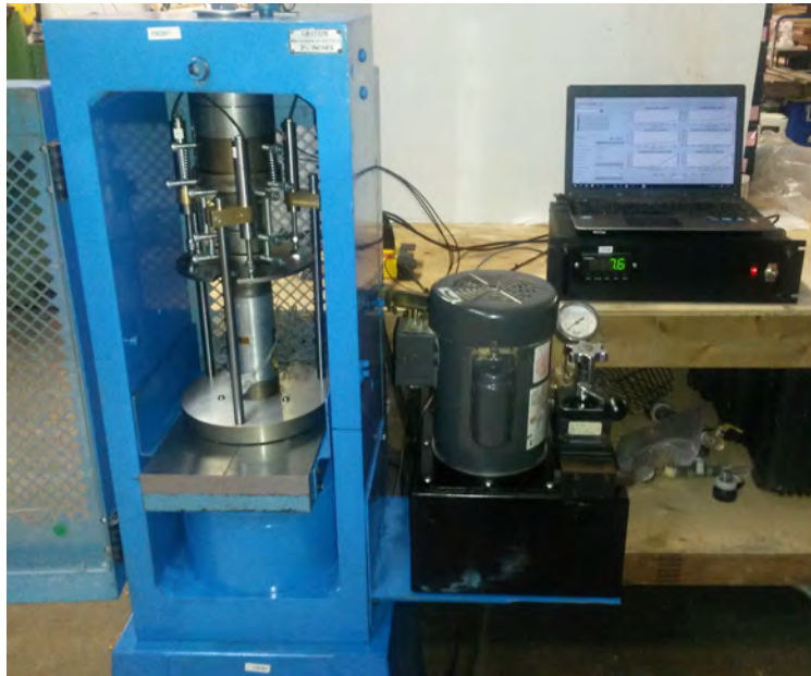
Figure 1: Forney loading frame setup for UCS testing.
