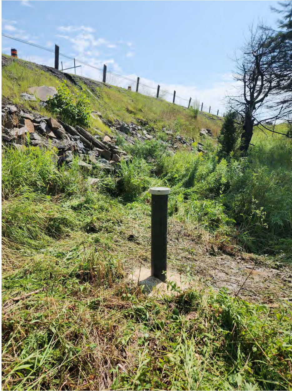
Photograph 5: Borehole 23-04 after completion.
