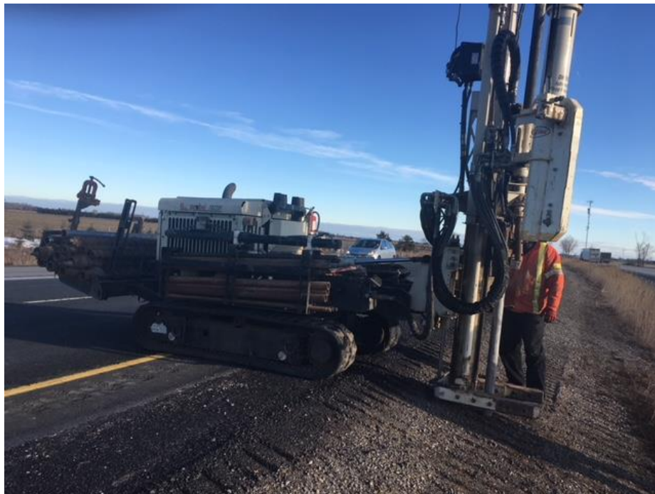
Photo 3. Rig used for drilling at Hwy 401, facing east
