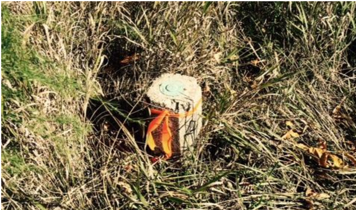
Photo 10: Temporary benchmark on MTO control point# 92
