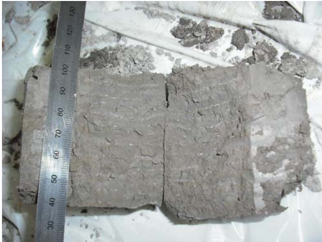
C15-3 Cut Section of Shelby Sample of Varved Clay
