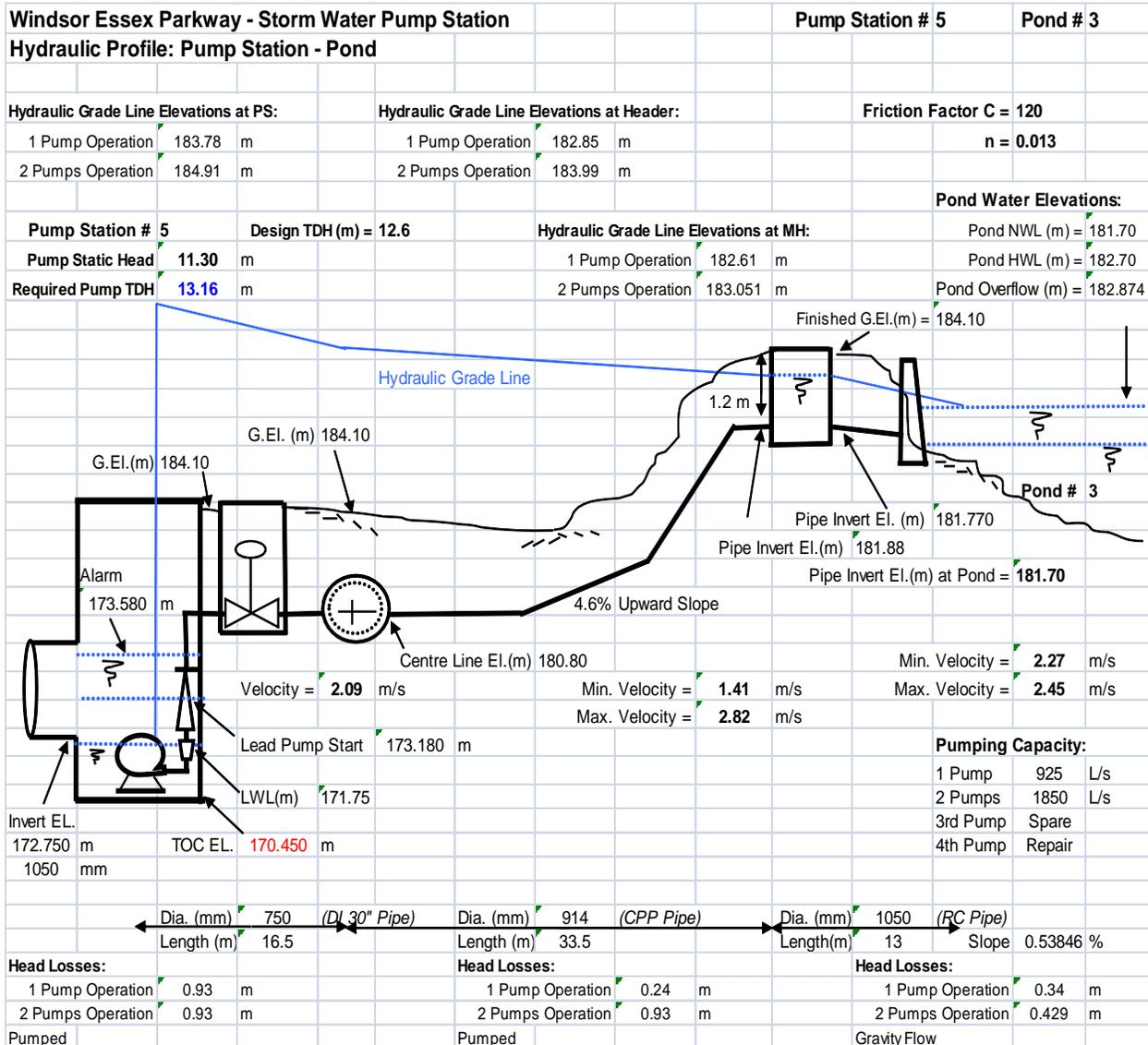
The following summarizes the maximum and minimum Static Head derived from the PS 5 hydraulic profile.
