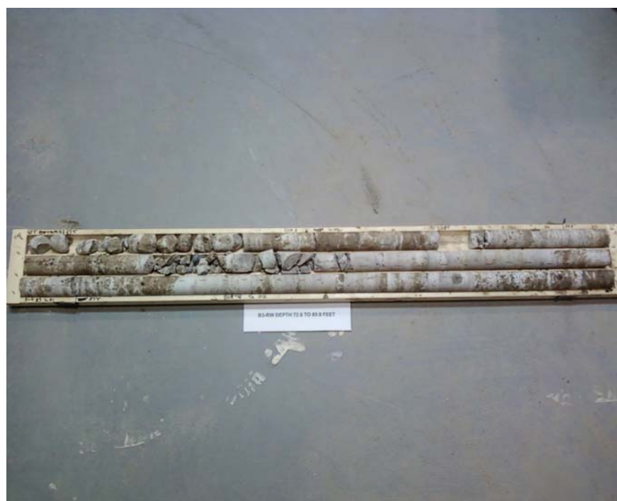
Photo 2 Borehole BH03-RW - Rock Core. Elevation 156.8 meters to 151.5 meters
