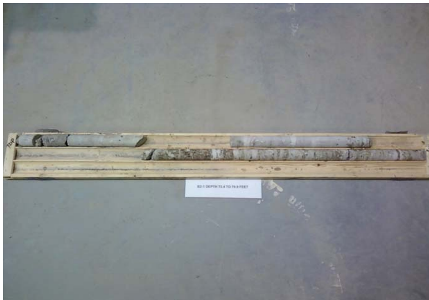
Photo 1: Borehole B2-1 - Rock Core. Elevation 156.2 meters to 154.2 meters
