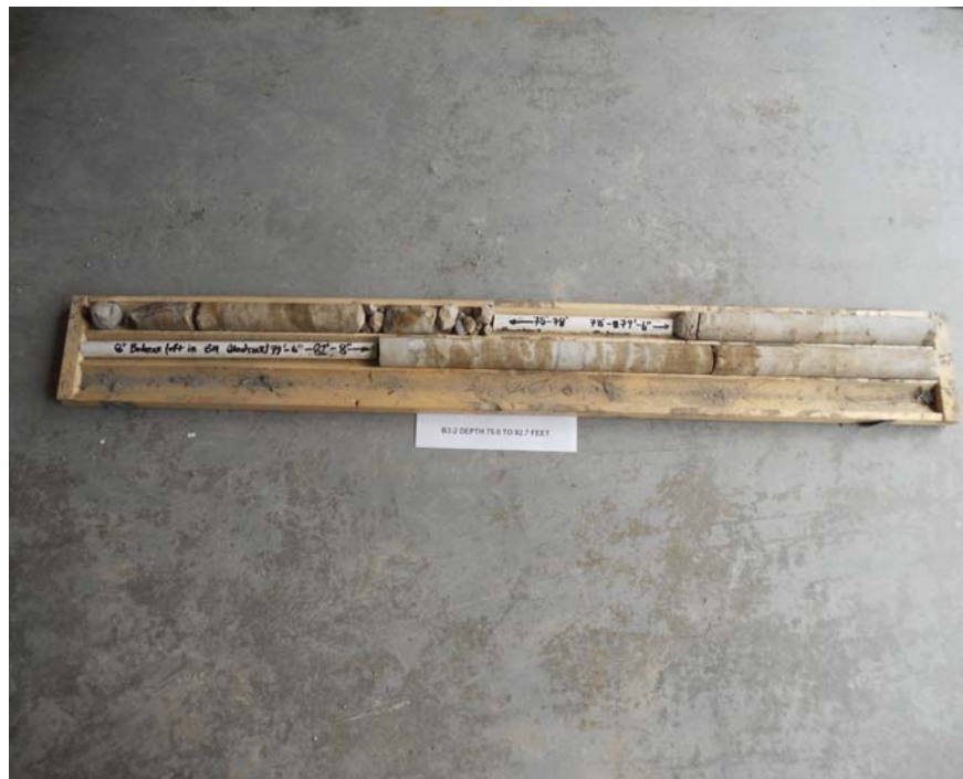
Photo 2 Borehole B3-2 - Rock Core. Elevation 156.0 meters to 153.6 meters
