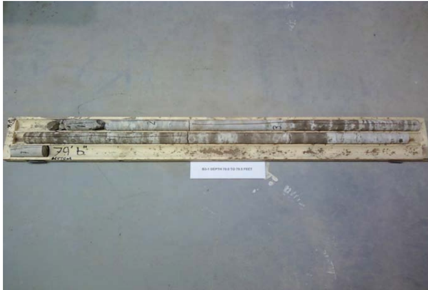
Photo 1: Borehole B3-1 - Rock Core. Elevation 157.6 meters to 154.7 meters
