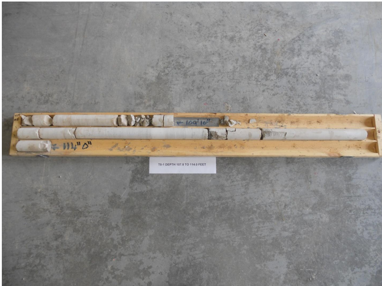
Photograph E-1: Borehole T8-1 – Rock Core Elevation 150.2 to 148.1 m
