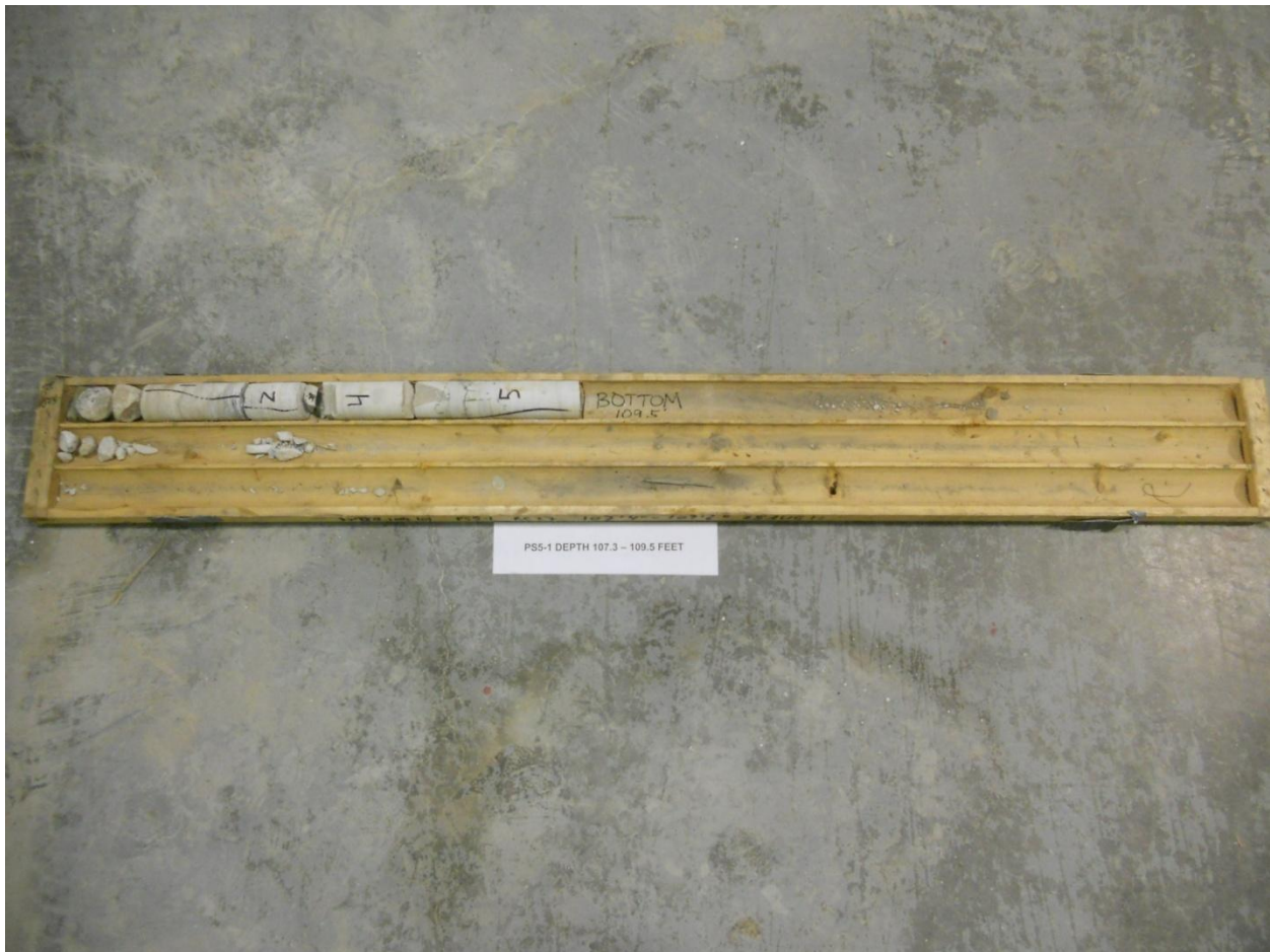
Photograph E-2: Borehole PS5-1 – Rock Core Elevation 150.1 to 149.3 m
