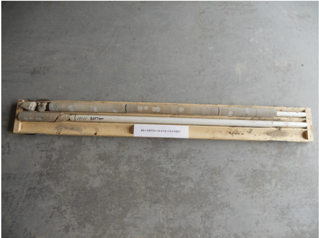
Photograph H-1: Borehole B9-1 – Rock Core Elevation 146.5 to 144.9 m
