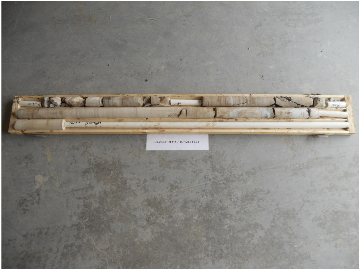
Photograph H-2: Borehole B9-2 – Rock Core Elevation 146.5 to 143.2 m
