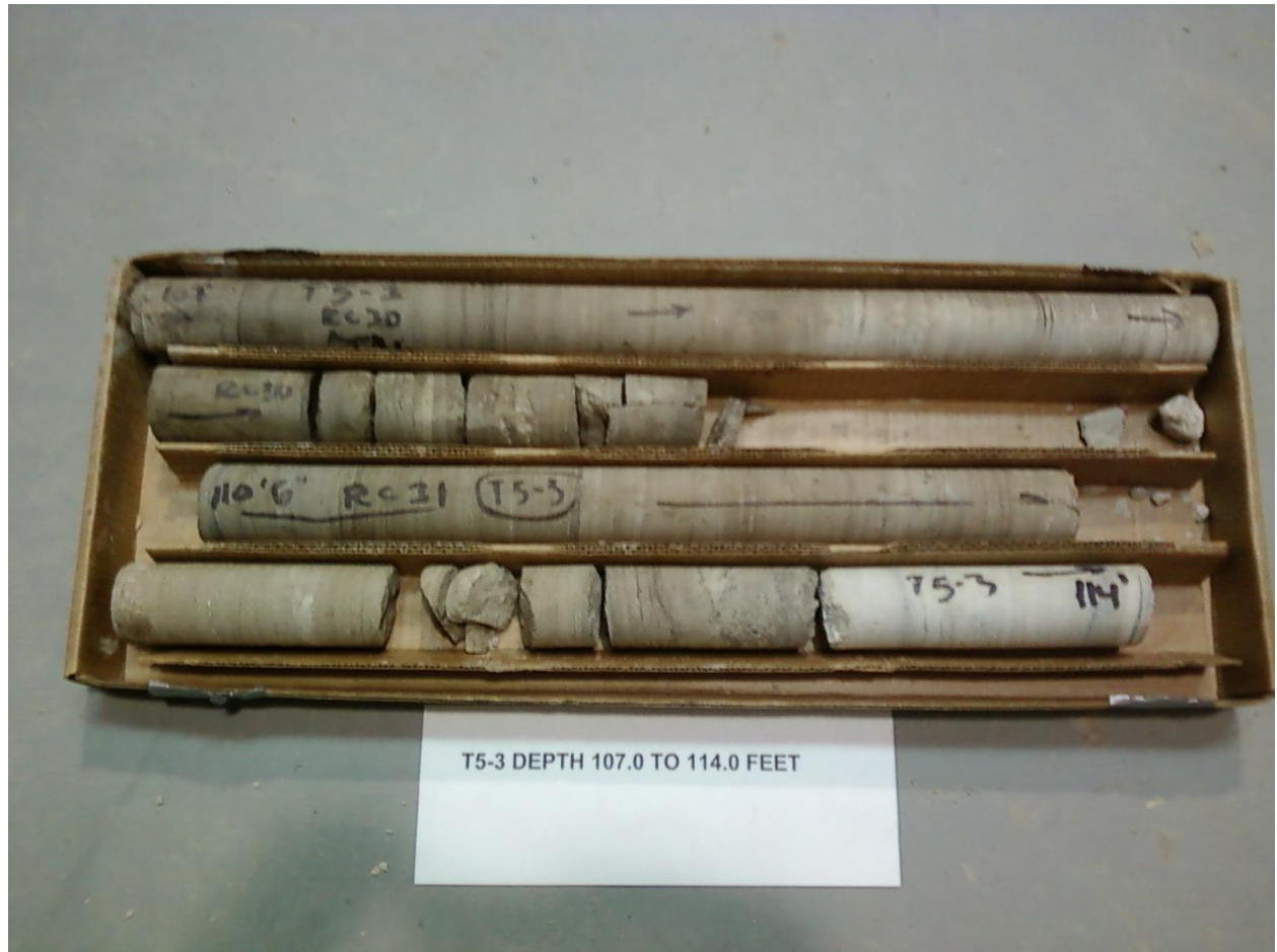
Photograph J-3: Borehole T5-3 – Rock Core Elevation 148.9 to 146.8 m
