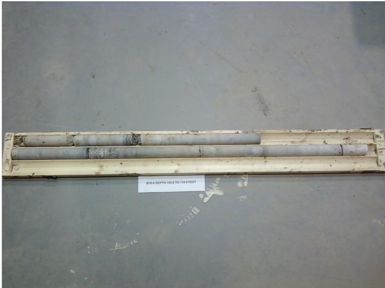
Photograph F-7: Borehole B10-6 – Rock Core Elevation 149.7 to 147.2 m
