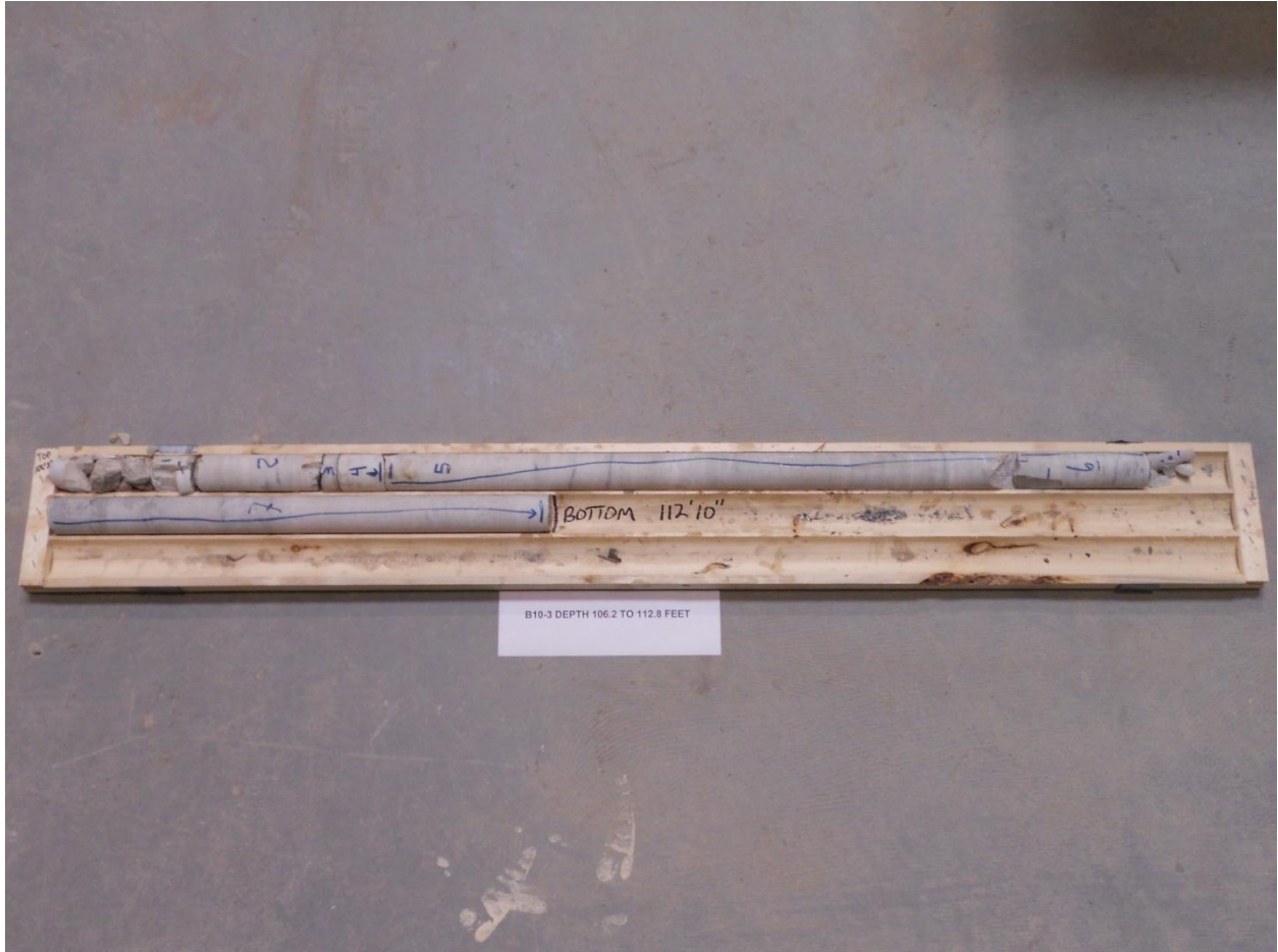
Photograph F-2: Borehole B10-3 – Rock Core Elevation 149.8 to 147.8 m
