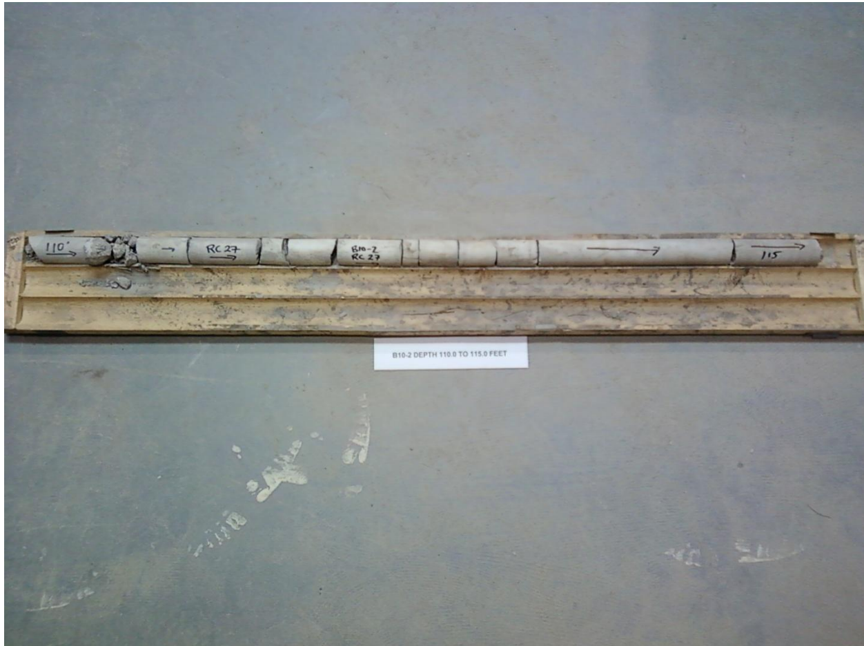
Photograph F-1: Borehole B10-2 – Rock Core Elevation 148.8 to 147.2 m
