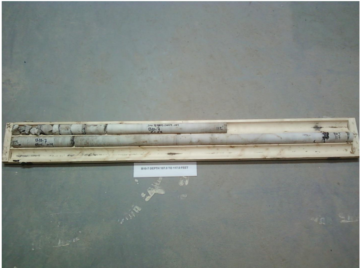
Photograph F-8: Borehole B10-7 – Rock Core Elevation 149.6 to 146.5 m
