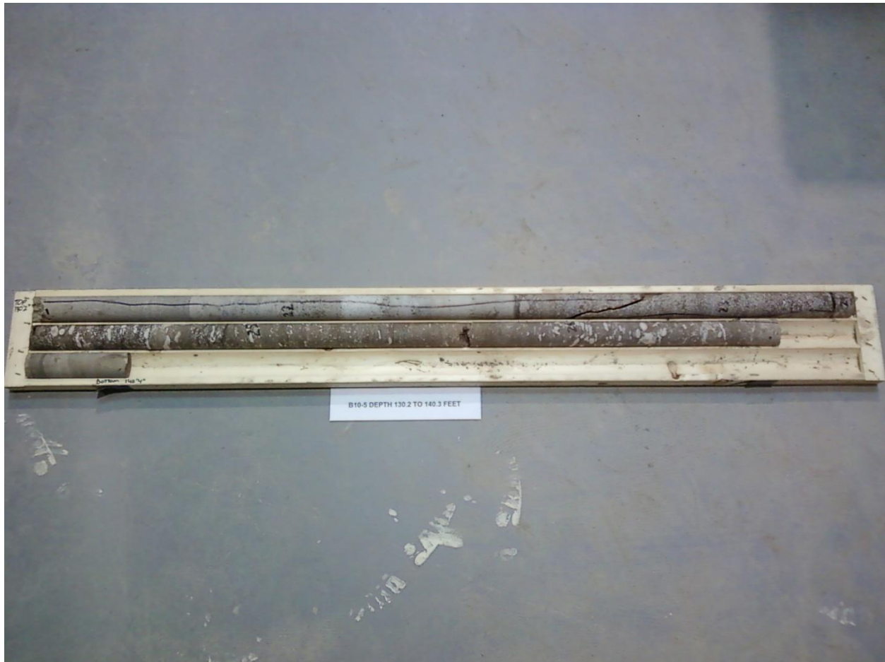
Photograph F-6: Borehole B10-5 – Rock Core Elevation 142.6 to 139.5 m
