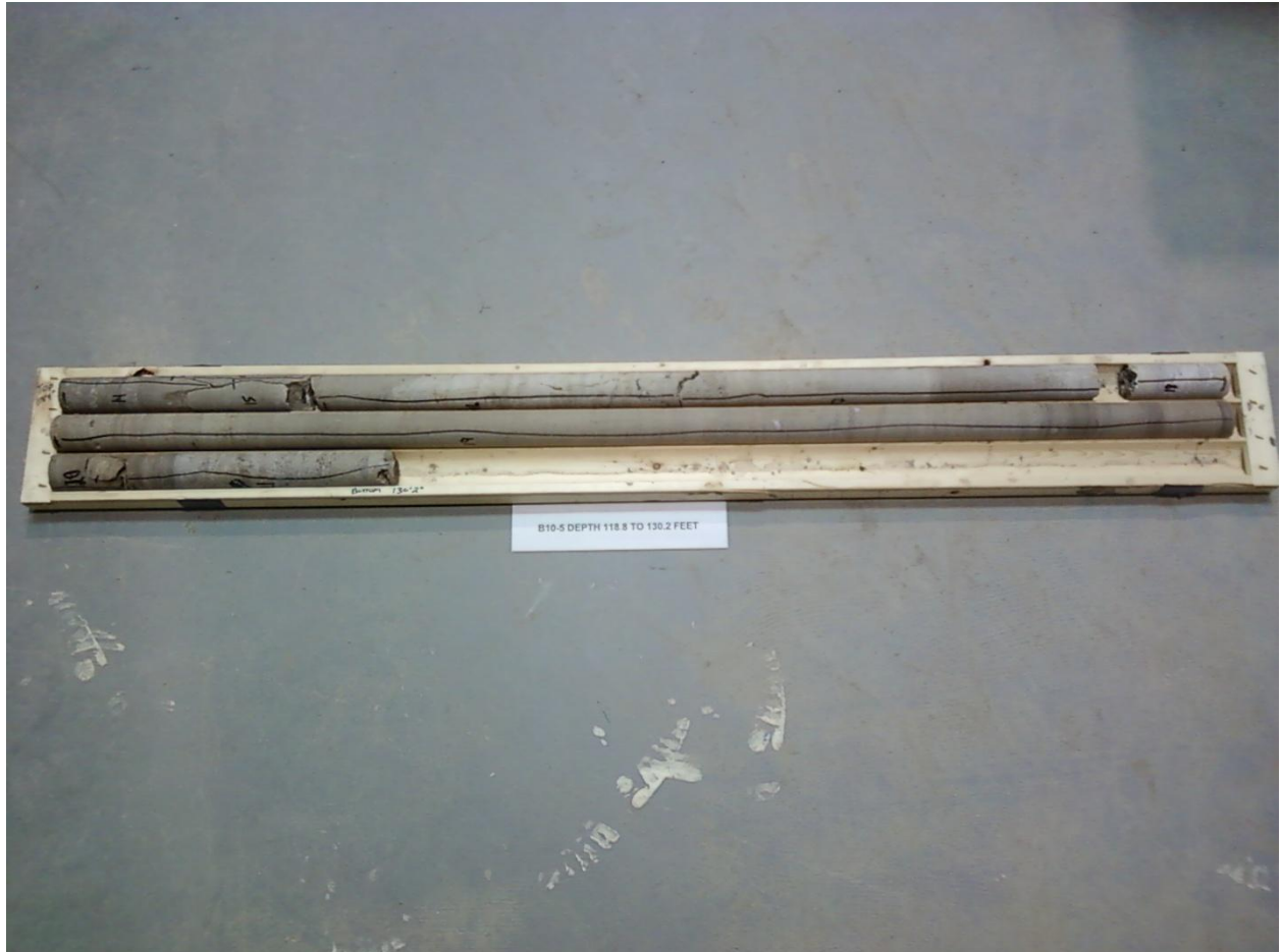
Photograph F-5: Borehole B10-5 – Rock Core Elevation 146.1 to 142.6 m
