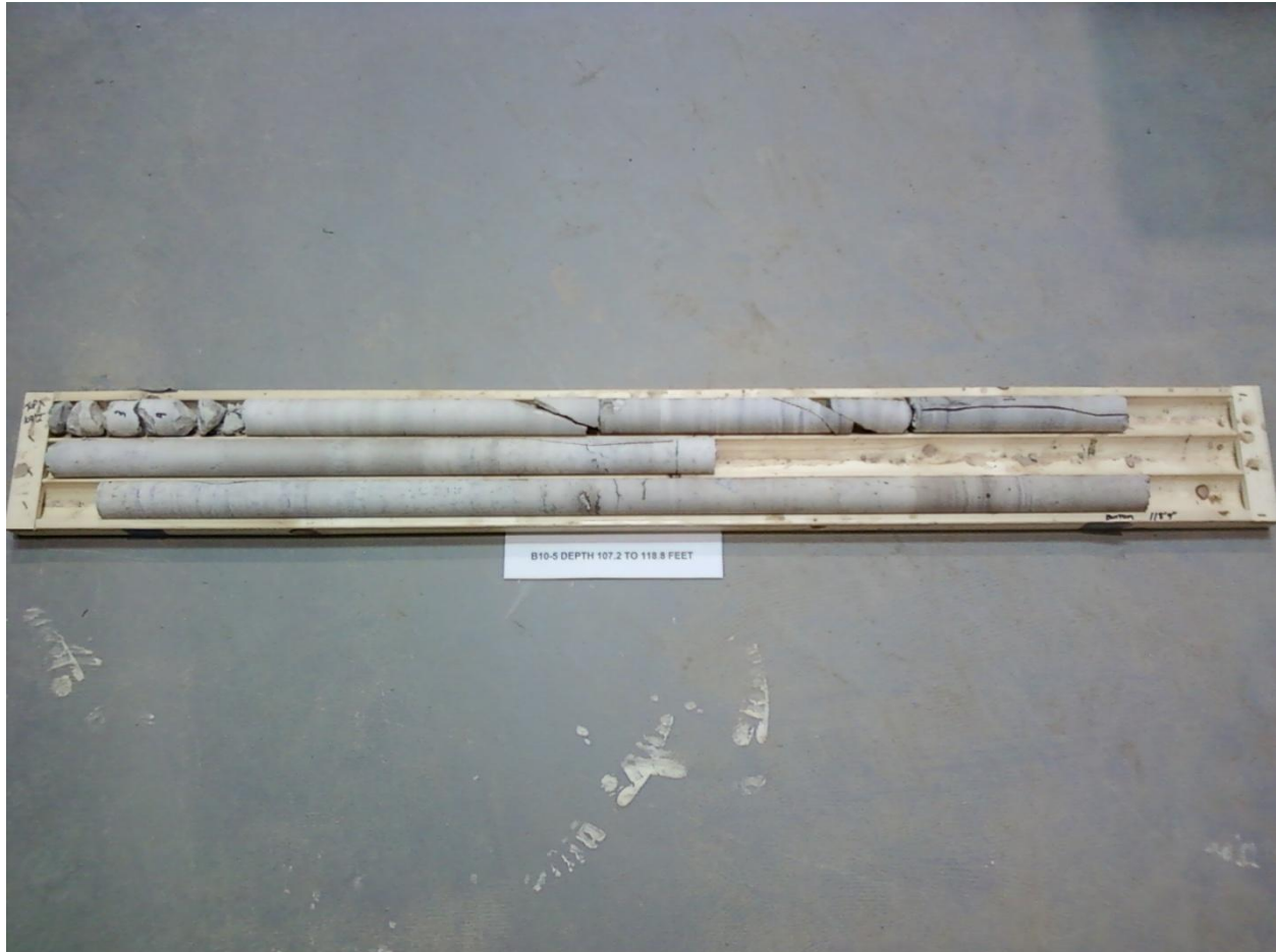
Photograph F-4: Borehole B10-5 – Rock Core Elevation 149.6 to 146.1 m
