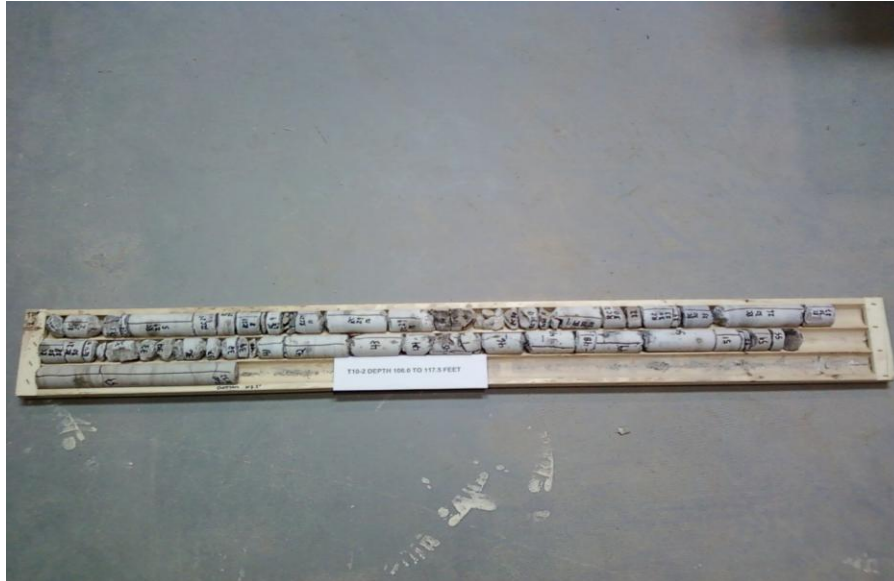
Photograph 1: Borehole T10-2 – Rock Core. Elevation 152.3 to 148.8
