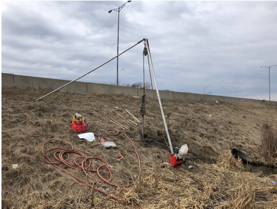
Photograph 3 – View of portable tripod equipment drilling at Borehole C6-01, west of inlet of Culvert 6
