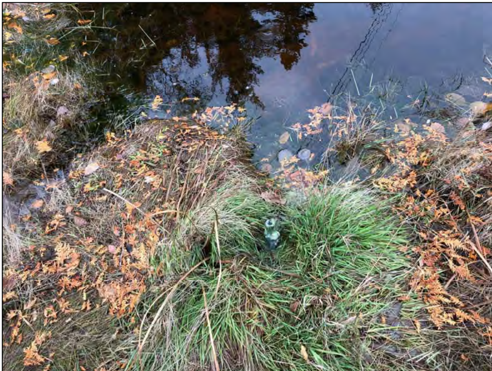
Photo 12: Piezometer installed in 1998 with active artesian flow [October 26, 2018]
