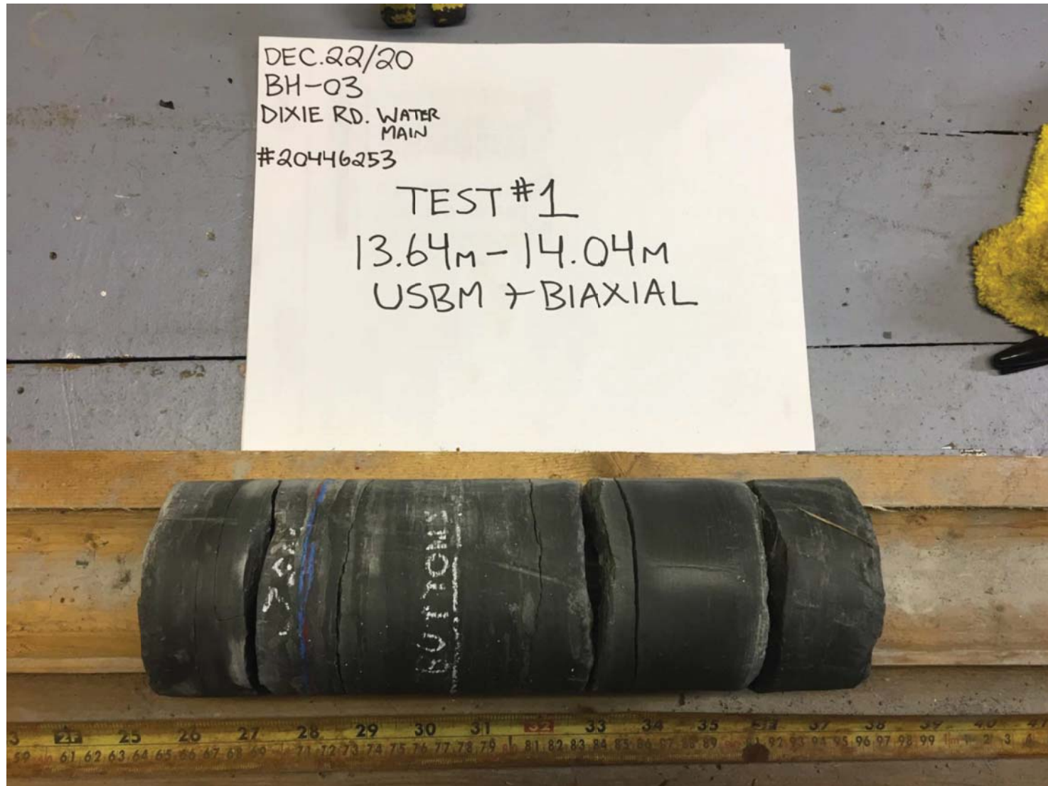
Figure A-2: Photograph of retrieved core for test BH-03-1 (13.6 m)
