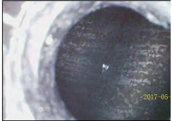
Photo 14 - V-2: Endoscope camera placed in the probe hole showing void.
