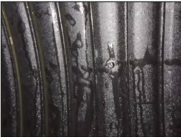
Photo 15 - V-3: Endoscope camera showing visible void.
