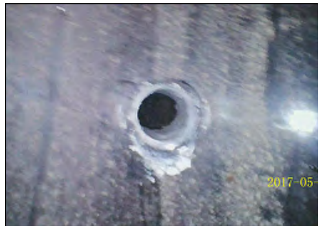
Photo 24 - V-5: Endoscope camera placed in the probe hole showing minor void.
