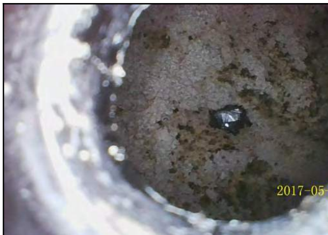
Photo 25 - V-6: Endoscope camera placed in the probe hole showing void.
