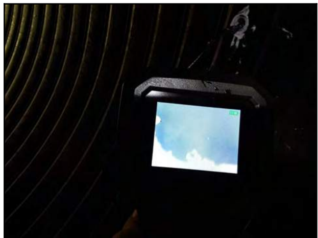
Photo 12 - V-1: Endoscope camera showing visible void.
