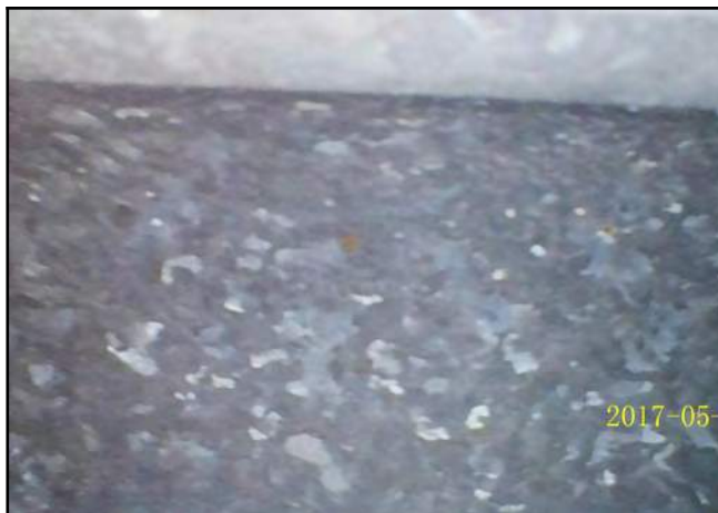
Photo 19 - V-3: Endoscope camera placed in the probe hole showing void.
