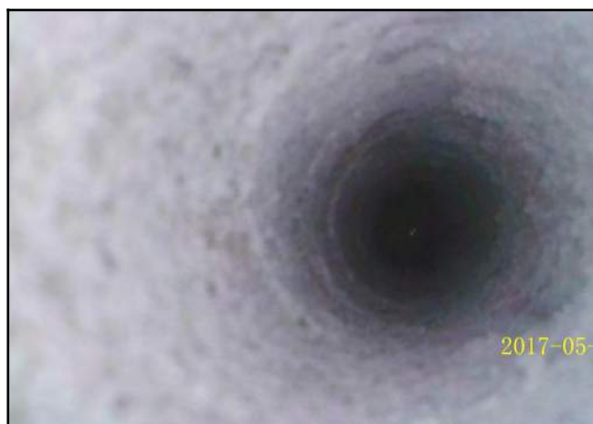
Photo 15 - V-1: Endoscope camera placed in the probe hole showing no void.
