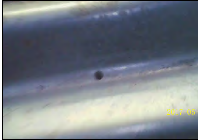
Photo 8 - V-1: Endoscope camera placed in the probe hole showing no void.
