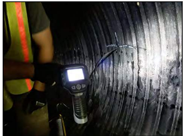
Photo 22 - V-5: Endoscope camera showing visible void.
