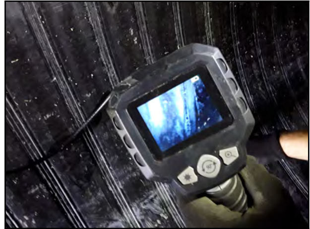
Photo 26 - V-6: Endoscope camera showing visible void.
