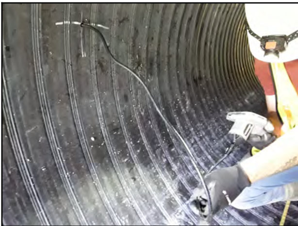
Photo 27 - V-6: Endoscope camera showing visible void.
