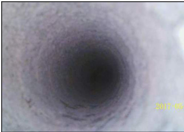
Photo 9 - V-1: Endoscope camera placed in the probe hole showing no void.
