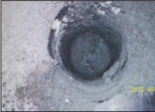
Photo 19 - V-3: Endoscope camera placed in the probe hole showing no void.
