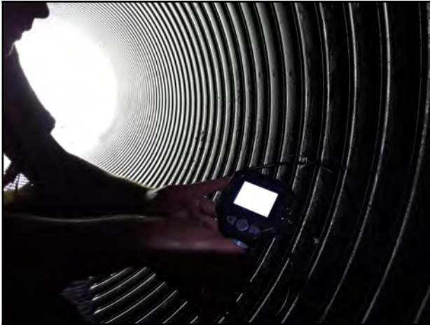
Photo 13 - V-2: Endoscope camera showing visible void.
