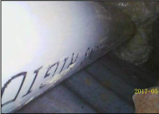
Photo 13 - V-1: Endoscope camera placed in the probe hole showing void.
