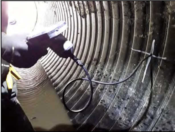
Photo 19 - V-3: Endoscope camera showing visible void.
