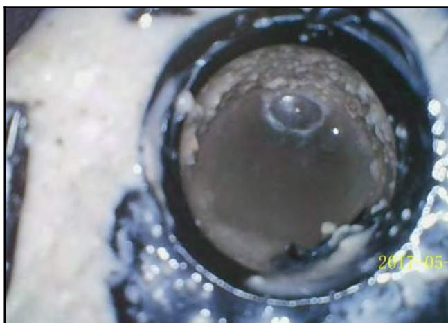
Photo 23 - V-5: Endoscope camera placed in the probe hole showing no void (control point).
