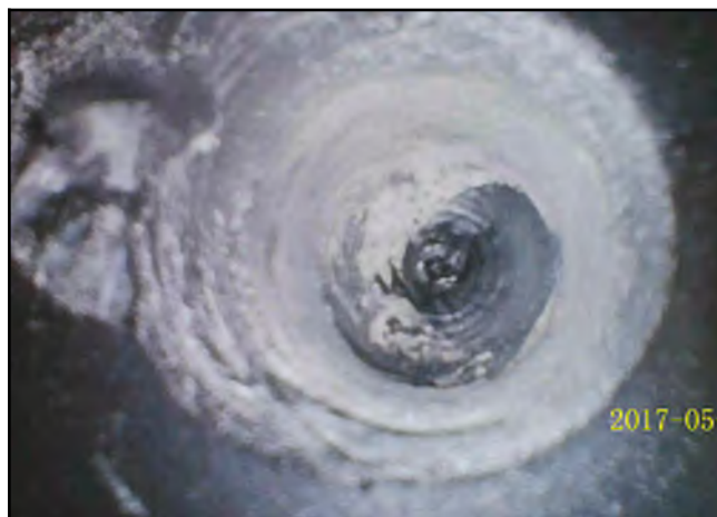
Photo 28 - V-7: Endoscope camera placed in the probe hole showing no void.
