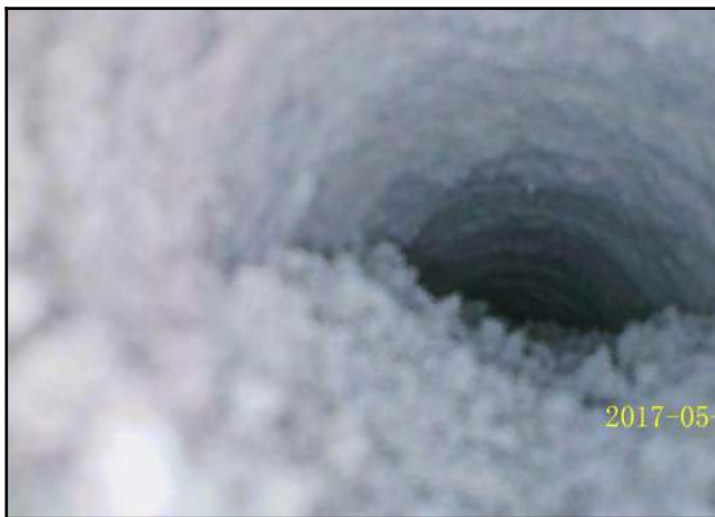
Photo 11 - V-3: Endoscope camera placed in the probe hole showing no void.
