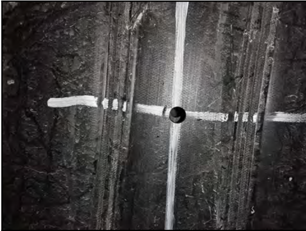
Photo 25 - V-5: Endoscope camera showing visible void.
