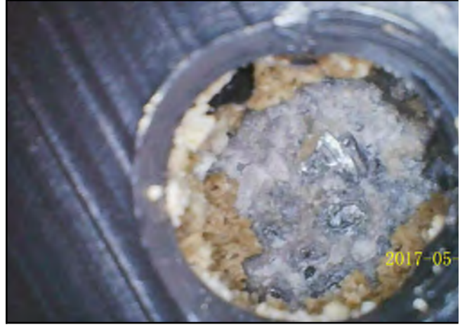
Photo 26 - V-7: Endoscope camera placed in the probe hole showing no void.
