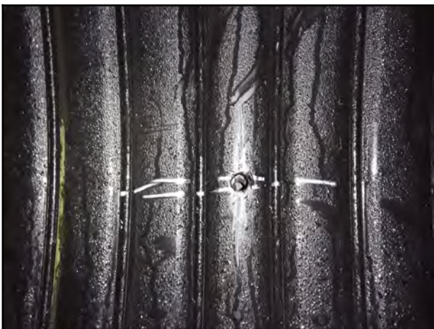
Photo 23 - 4 m at 8:30 with visible void.
