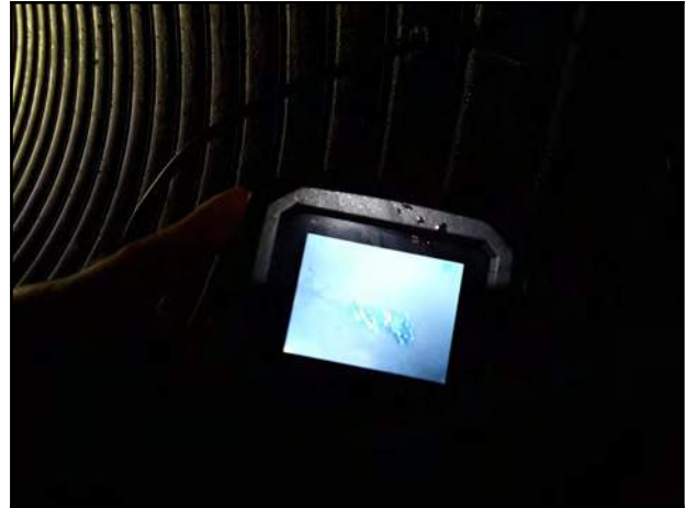
Photo 14 - V-2: Endoscope camera showing visible void.
