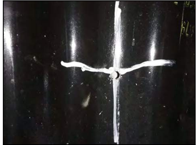
Photo 26 - V-5: Endoscope camera showing visible void.
