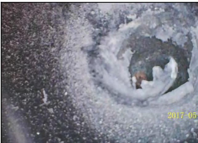
Photo 23 - V-5: Endoscope camera placed in the probe hole showing no void.
