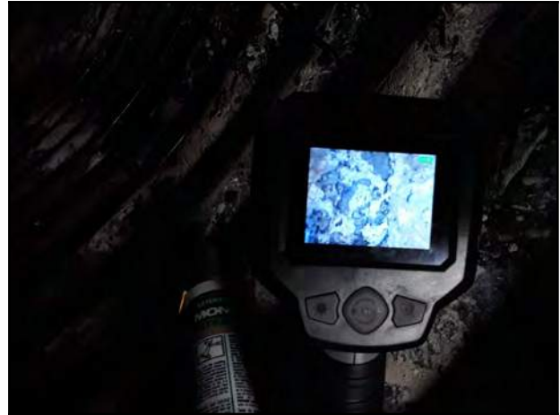
Photo 20 - V-3: Endoscope camera showing visible void.
