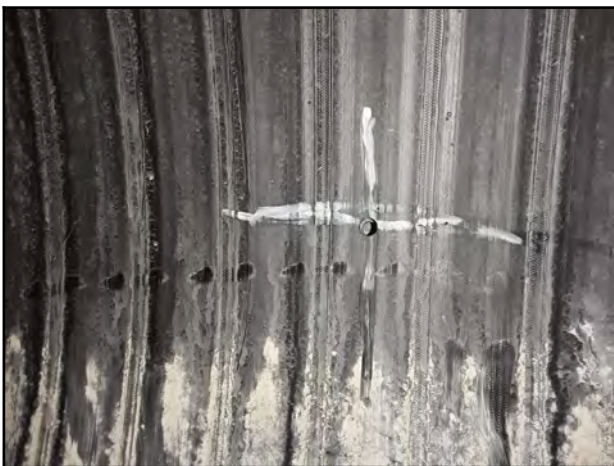
Photo 23 - V-5: Endoscope camera showing visible void.
