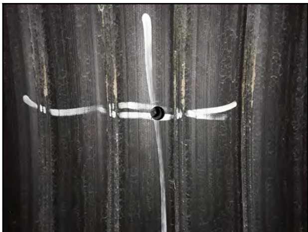
Photo 19 - V-5: Endoscope camera showing visible void.
