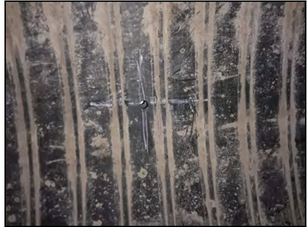
Photo 14 - V-1: Endoscope camera showing visible void.
