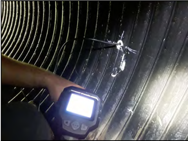
Photo 19 - V-4: Endoscope camera showing visible void. Image is blurry, difficult to see void.
