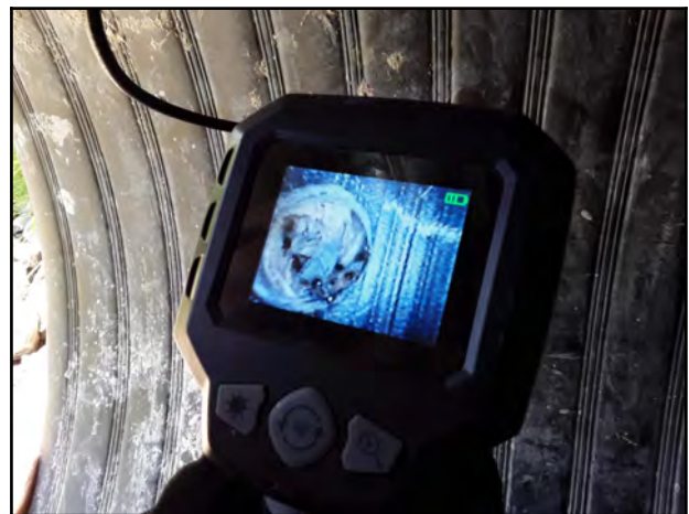
Photo 12 - V-1: Endoscope camera showing visible void.
