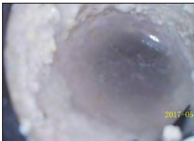
Photo 24 - V-5: Endoscope camera placed in the probe hole showing no void (control point).
