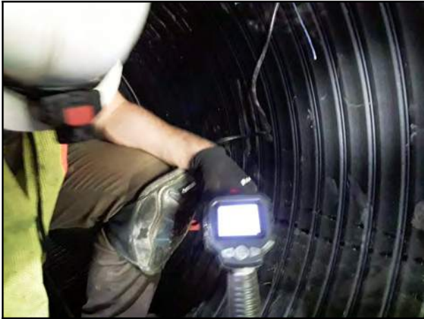
Photo 25 - V-6: Endoscope camera showing visible void.
