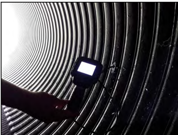
Photo 11 - V-1: Endoscope camera showing visible void.
