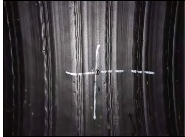
Photo 20 - V-4: Endoscope camera showing visible void.
