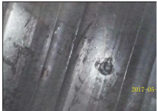
Photo 12 - V-1: Endoscope camera placed in the probe hole showing void.
