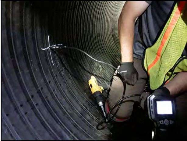
Photo 19 - V-4: Endoscope camera showing visible void.
