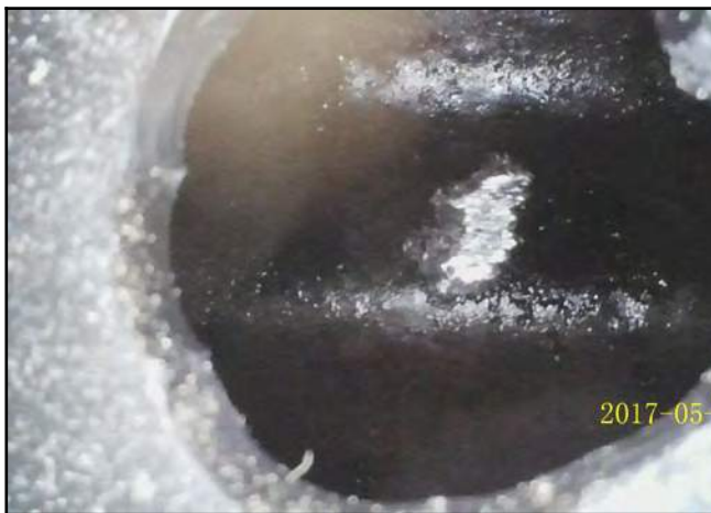
Photo 17 - V-3: Endoscope camera placed in the probe hole showing void.
