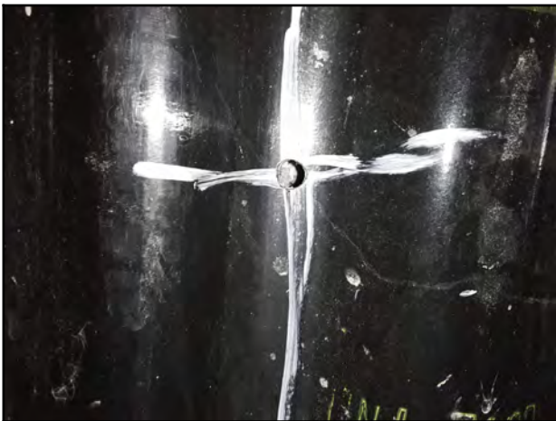
Photo 21 - V-3: Endoscope camera showing visible void.
