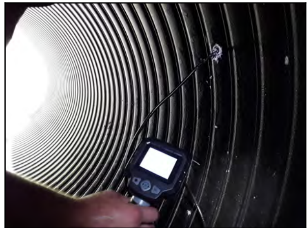
Photo 16 - V-3: Endoscope camera showing visible void.
