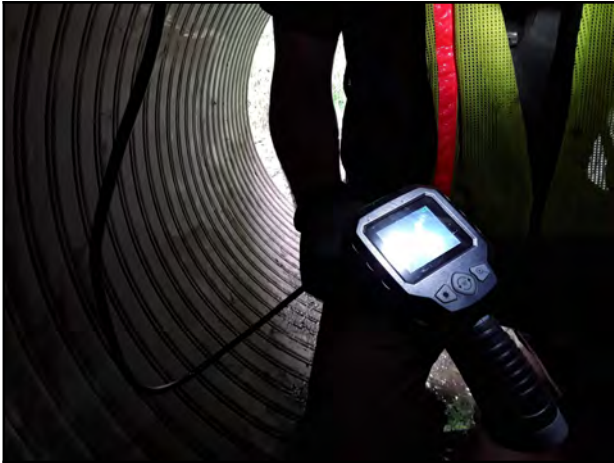
Photo 13 - V-1: Endoscope camera showing visible void.
