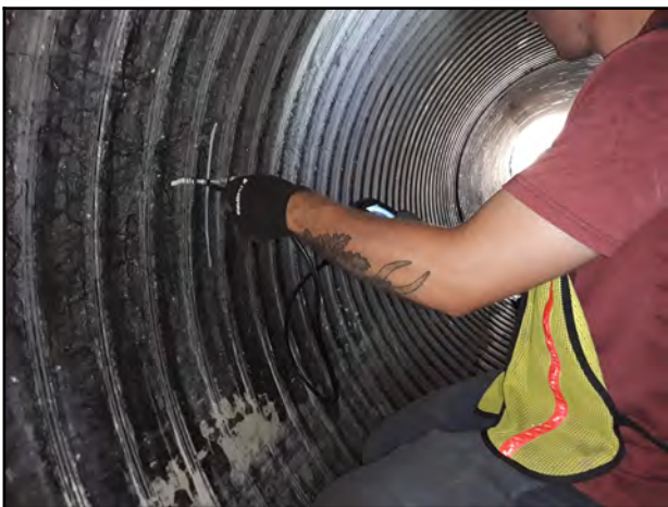
Photo 23 - V-5: Endoscope camera showing visible void.
