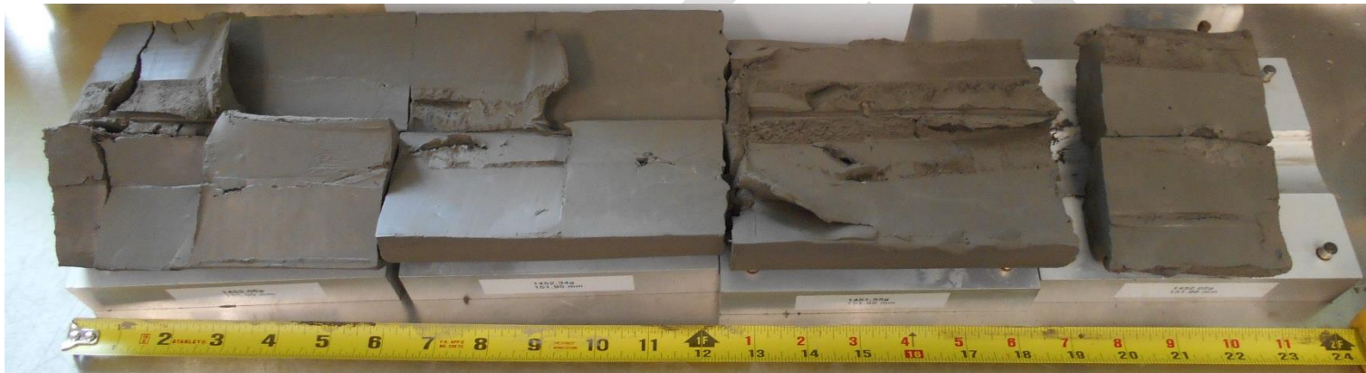
Photo C.1. Shelby tube sample TW7 @ 5.3 to 5.9 m from Borehole 17-4
